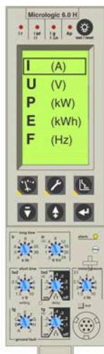
Figure 37 - MicroLogic Type H Trip Unit
