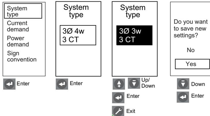
9. Do not use “3-phase, 4-wire, 4 CT” type unless neutral is effectively connected to the trip device (neutral voltage connection is external to the 3-pole circuit breaker). (See neutral CT instruction bulletin.)
