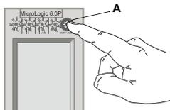
Do not return circuit breaker to service until cause of trip is determined. For more information, refer to the circuit breaker installation instructions shipped with the circuit breaker.
