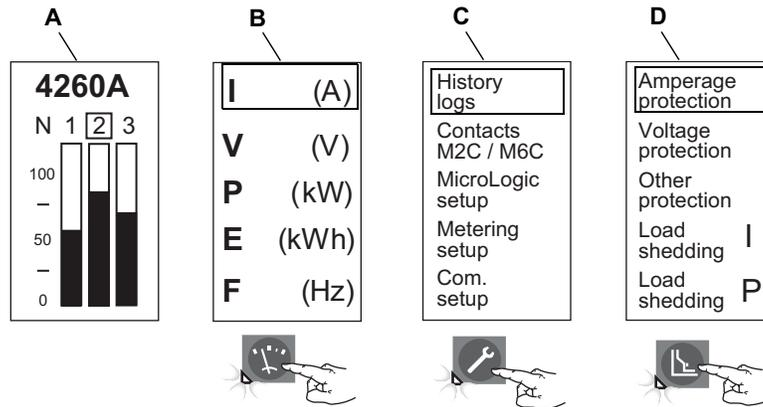
The MicroLogic P trip unit has a default bar graph display of currents and three different menus which can be accessed using navigation buttons:
