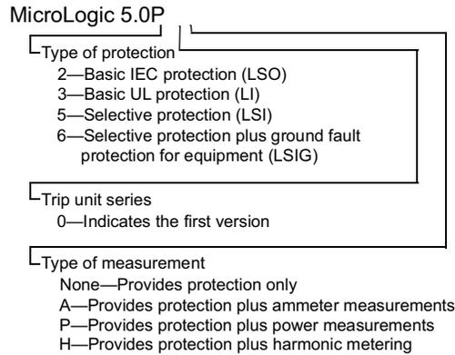
MicroLogic trip units are field replaceable to allow for upgrading of the trip unit in the field. For complete information on available circuit breaker models, frame sizes, interrupting ratings, sensor plugs, rating plugs and trip units, see the product catalog.
