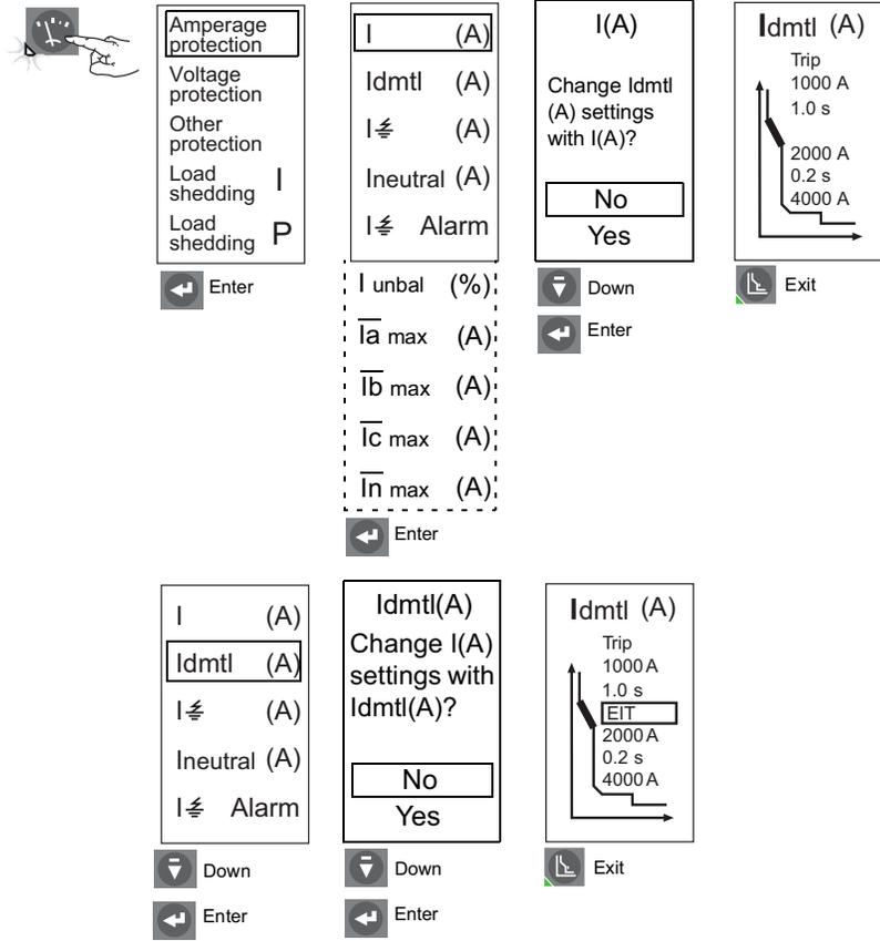
**Figure 84 - Check Amperage Protection**
