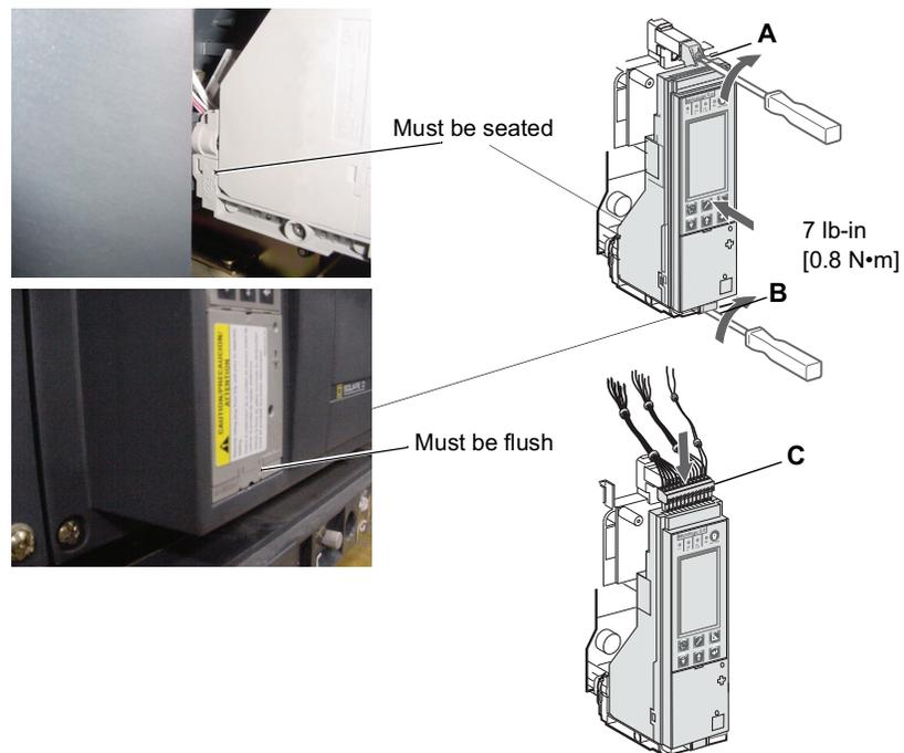
9. Install adjustable rating plug into the trip unit.
