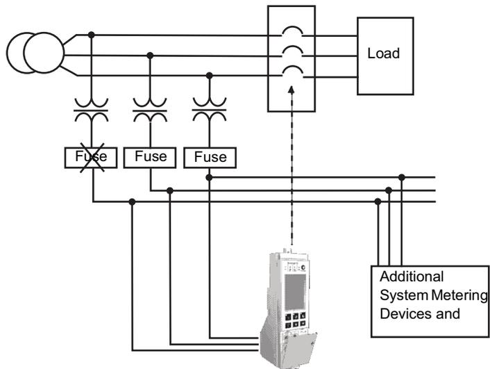
**Figure 108 - Circuit Configuration 4**
