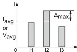
$$I_{avg} = \frac{I_a + I_b + I_c}{3} \quad V_{avg} = \frac{V_a + V_b + V_c}{3}$$
