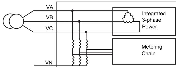
**Figure 104 - Open Phase on Three-phase Power Supply**
