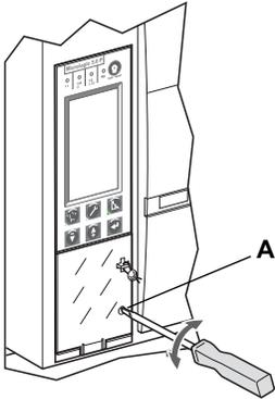
Paragraph 230-95 (c) of the National Electrical Code requires that all equipment ground-fault protection systems be tested when first installed.
