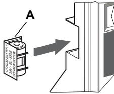
**NOTE:** Battery holder with battery is located under the side flap in the cardboard box the trip unit is shipped in.
