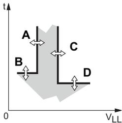
Provides pickup and dropout values for alarm, contacts or tripping for current and voltage values. (There is no minimum for current.)
