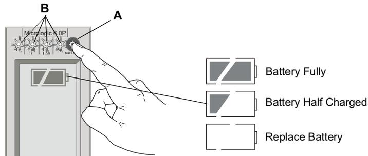
3. If the battery bar graph shows the battery needs to be changed, use Square D battery catalog number S33593:
