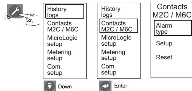
1. Enter M2C/M6C contacts alarm type into trip unit memory. Available alarms are:
