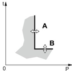
Reverse power protection protects alternators against absorption of the total actual power over all three phases in the event that a drive motor fails.
