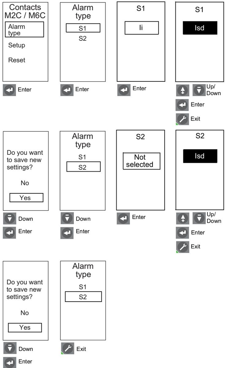
2. Set up M2C/M6C contact alarm mode. Contact modes available are:
