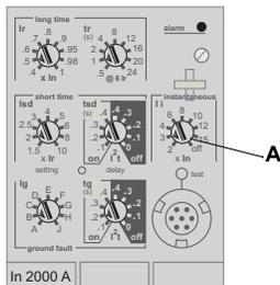
Instantaneous protection protects equipment against short circuits with no intentional time delay.
