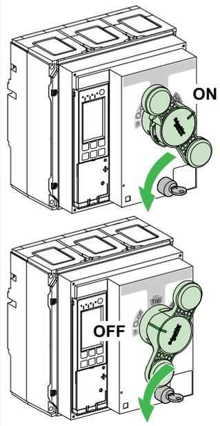
The diagram consists of two parts. The top part shows a circuit breaker with its handle in the 'ON' position, indicated by a green arrow pointing to the right and the word 'ON' next to it. The bottom part shows the same circuit breaker with its handle in the 'OFF' position, indicated by a green arrow pointing to the left and the word 'OFF' next to it. The handle is a green, T-shaped lever with a keyhole at the bottom. |
