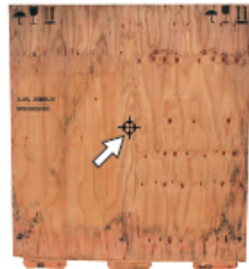
Figure 16 Centre of Gravity Information on the Transport Unit (wooden crate for export packaging)
