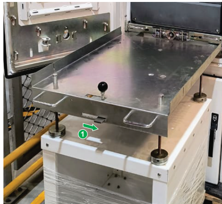
Figure 23 Turning Lever on Trolley to the Left
