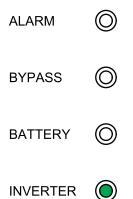
**NOTE:** If autostart is disabled, the inverter and bypass will not restart automatically. From the home screen on the display select **Control > Inverter ON/OFF > Turn Single INV ON**.
