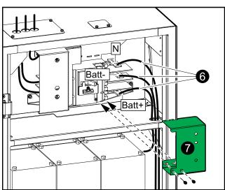
7. Install the protection cover over the terminals on the right side of the battery breaker.
