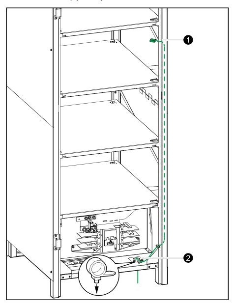
2. Route the battery temperature sensor cables through the top or the bottom of the empty battery cabinet to the UPS dry contact terminals BAT\_T for Easy UPS 3M and J12 for Easy UPS 3L.
