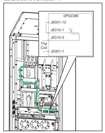
8. Note the terminal locations for the input power cables (single mains configuration) or bypass power cables (dual mains configuration).
