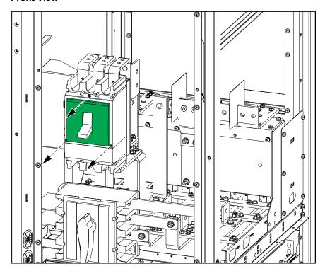
b. Remove the cover from the signal connection terminals.
