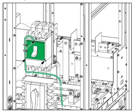
10. Install the new front plate (TME11303) from the backfeed kit on the UPS with the eight M6 screws (803-8170) removed in step 2. Reinstall the cover over the signal connection terminals.
