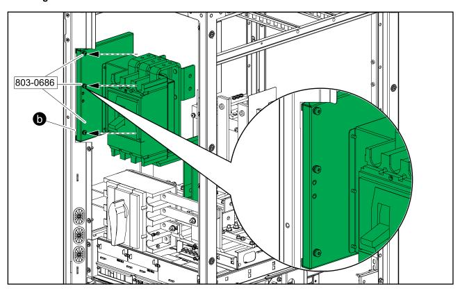
c. Fasten the three backfeed busbars with the six M8 nuts (803-8007) removed in step 5.
