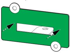
b. Install the PCBA board on the front bracket and fasten with the screw provided. Torque to 0.49 Nm (0.37 lb-ft/4.33 lb-in).
