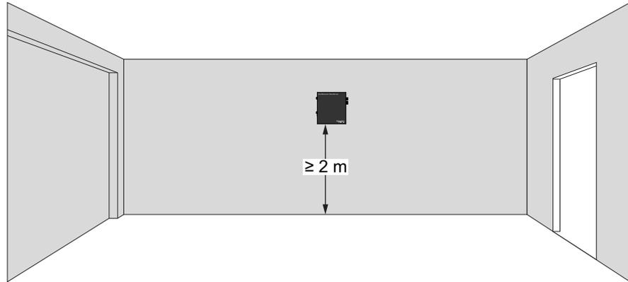
1. Mark the positions of three drilling holes on the surface to install the mounting bracket.
