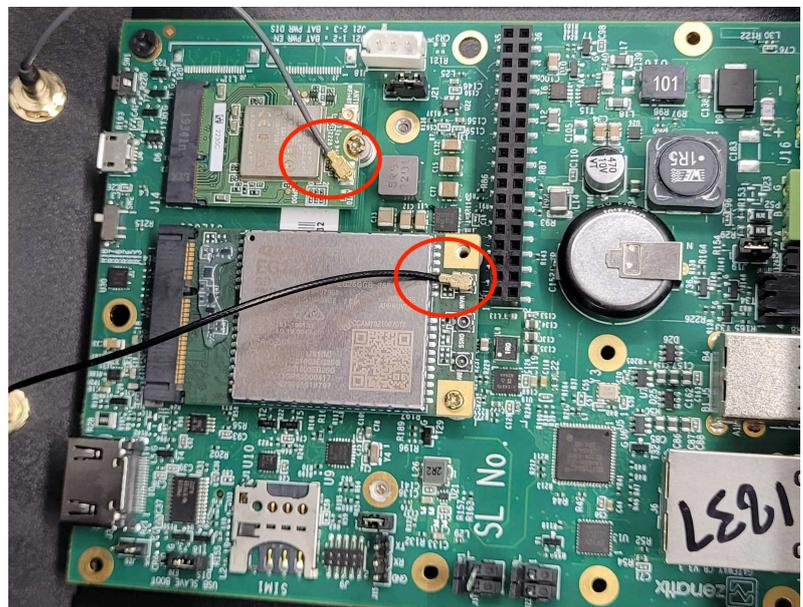
(3) Attach the antenna wire again to the **MAIN** connection point.
