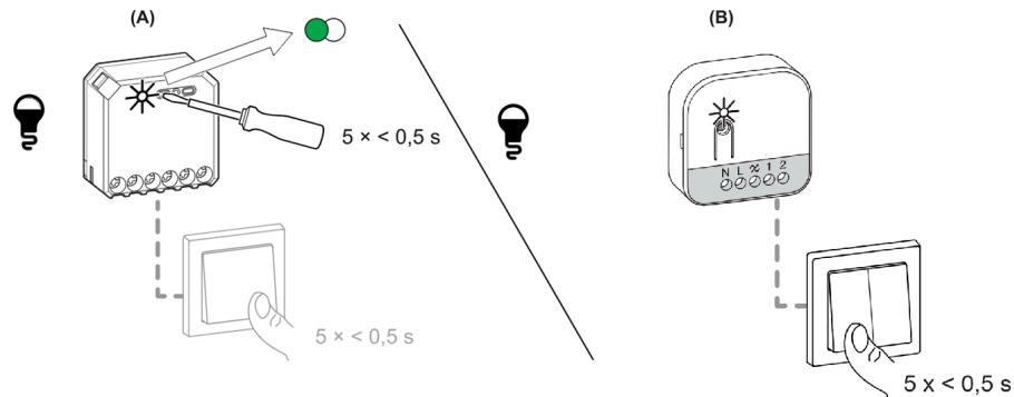
The status LED blinks green on the micro module LED.
