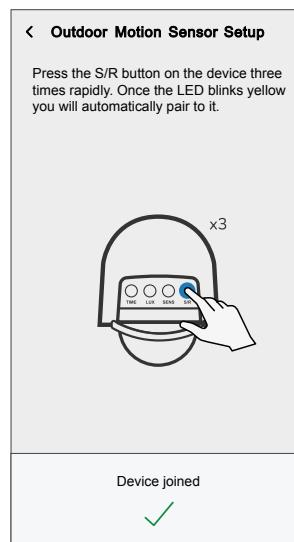
5. Mount the motion sensor on the wall or ceiling and tap **Next** to start configuring the motion sensor.
