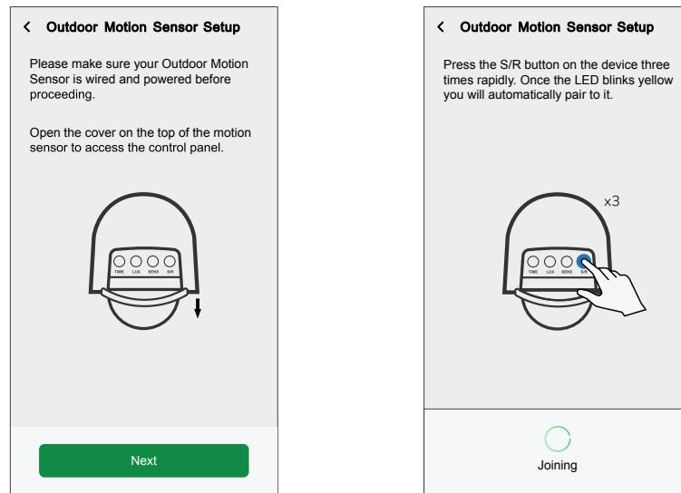
The app confirms that the device is joined and a yellow LED blinks on the motion sensor.
