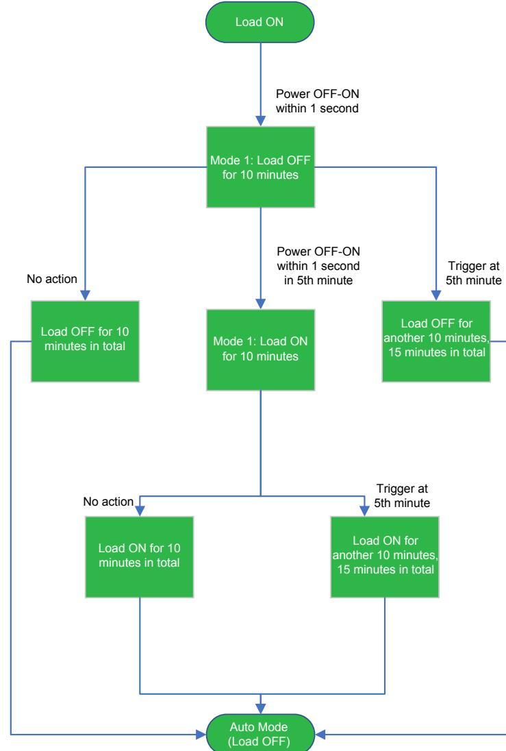
**To manually exit mode 1:** Switch to mode 2 (power OFF - ON twice within 2 s), then power OFF-ON within 1 s.
