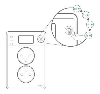
The push-button enables you to switch between Guide light, Night light and OFF modes.
