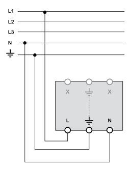
The wall-insert has three screwless terminals at the bottom – Live (L), Neutral (N) and Earth ( $\pm$ ) with a 2-wire entry for each terminal.
