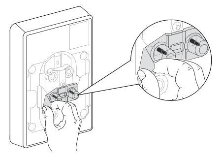
**NOTE:** Any damage to the contact pins; for example, bending, breaking, or deformation, will interfere with the functioning of the product.
