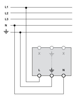
The wall-insert has three screwless terminals at the bottom – Live (L), Neutral (N) and Earth ( $\pm$ ) with a 2-wire entry for each terminal.
