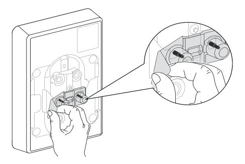
**NOTE:** Any damage to the contact pins; for example, bending, breaking, or deformation, will interfere with the functioning of the product.
