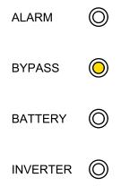
4. Wait approximately 20 seconds until inverter LED turns steady green, the UPS transfers automatically from static bypass mode to normal mode.
