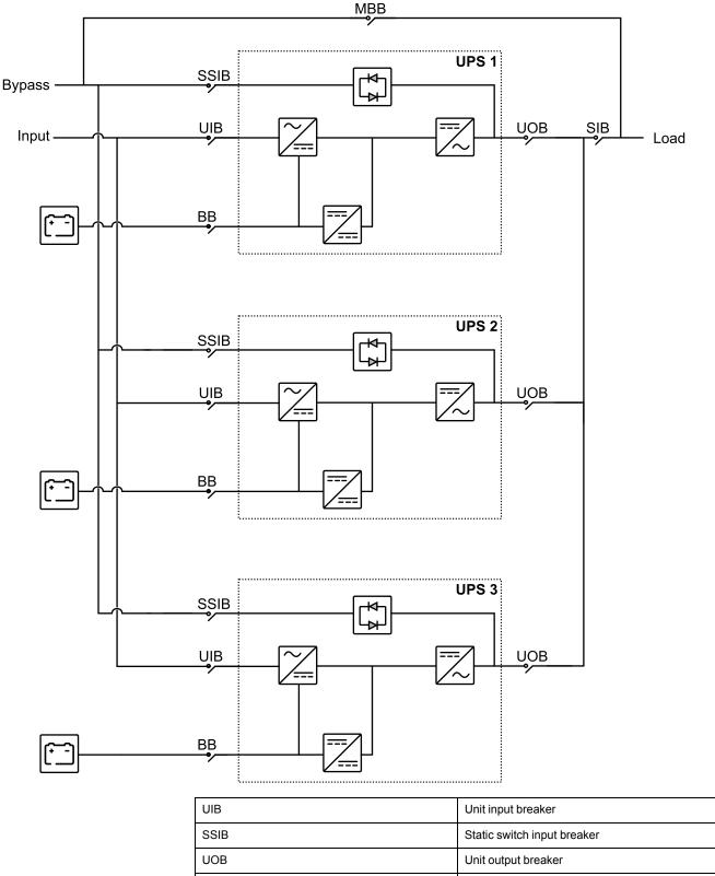
MBB Maintenance bypass breaker SIB System isolation breaker ВВ Battery breaker
