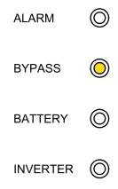
5. Wait approximately 20 seconds until inverter LED turns steady green, the UPS transfers automatically from static bypass mode to normal mode.
