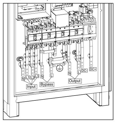
5. On the static switch input breaker SSIB, push the button to set the static switch input breaker SSIB from the OFF (open) position to the Trip position.
