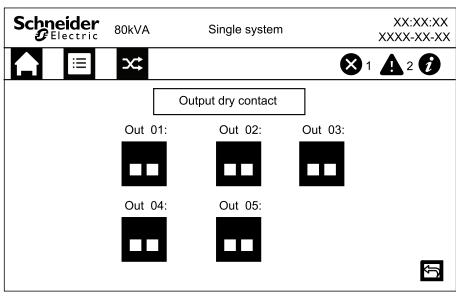
4. Set the **Status** of the output dry contact to **Closed** and the **Function** to **Backfeed on bypass**.
