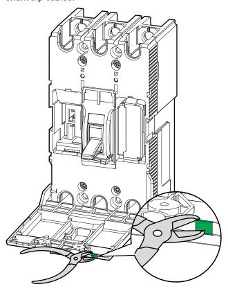
10. Close the unit input breaker UIB cover. Route the backfeed shunt trip cables through the top notch.
