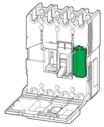
9. Make a notch in the top of the static switch input breaker SSIB cover for the backfeed shunt trip cables.
