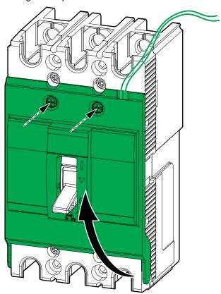
11. Tighten the indicated screws and torque to 1 Nm.
