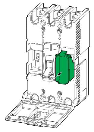
9. Make a notch in the top of the unit input breaker UIB cover for the backfeed shunt trip cables.
