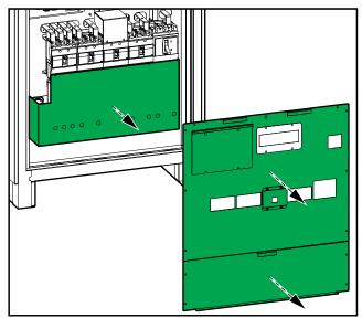
4. Measure for and verify ABSENCE of voltage on each input/bypass/output busbar before continuing.
