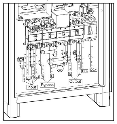
5. On the unit input breaker UIB, push the button to set the unit input breaker UIB from the OFF (open) position to the Trip position.
