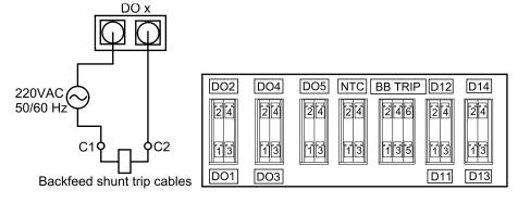
14. Route the backfeed shunt trip cables along the post cables reliefs and into the bottom brush plates to the output busbars (L, N).
