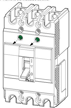
7. Open the unit input breaker UIB cover. The backfeed kit will be installed in the marked position.
