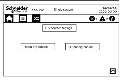
3. Select the output dry contact for configuration that you connected the backfeed shunt trip cables to during installation.
