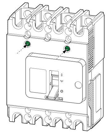
7. Open the static switch input breaker SSIB cover. The backfeed kit will be installed in the marked position.
