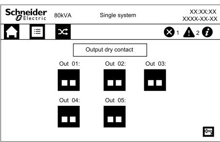
3. Set the **Status** of the output dry contact to **Closed** and the **Function** to **Backfeed on input**.
