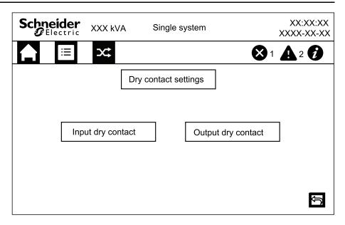
2. Select the output dry contact for configuration that you connected the backfeed shunt trip cables to during installation.
