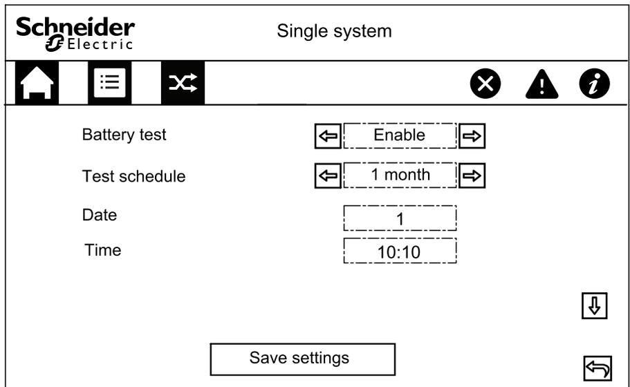
2. Select if **Battery test** should be performed automatically. If this function is enabled, configure the following settings:
