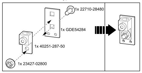
3. Install the mechanical lug assembly on the top and/or bottom of the neutral busbars with the provided screws.
