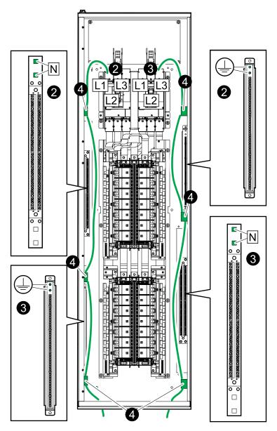
**NOTE:** The maximum allowed neutral cable size is 350 kcmil with the preinstalled cable lugs. For >350 to <500 kcmil neutral cable, replace the preinstalled neutral cable lug with kit TME69214, see Install the Neutral Mechanical Cable Lug Kit TME69214 (Option), page 25 for details.
