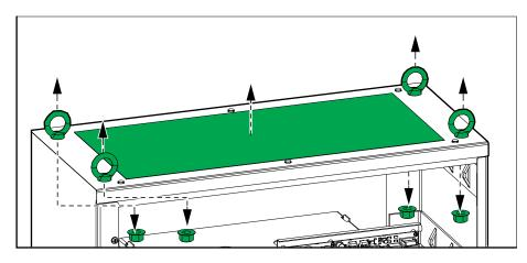
7. Install the top gland plate (removed during unpacking of the cabinet).
