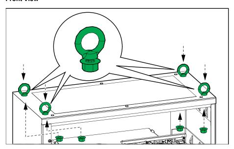
12. Attach lifting equipment to the eye bolts. This will prevent the cabinet from tipping over when the cabinet is no longer mounted to the wall/floor.
