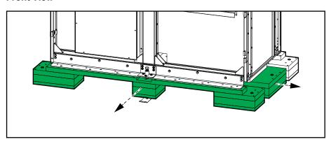
12. Use a drilling machine or a wrench to turn the jack to lower the cabinet down onto the floor. Turn the jack until it can be removed from the front transportation bracket.
