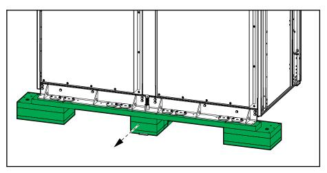
16. Remove the rear transportation bracket, the jack (TME72611) and the floor protection plate (TME48195) from the cabinet. Save the rear transportation bracket and the screws, the rear transportation bracket is reused for seismic anchoring. See the installation manual for details.
