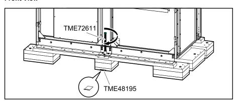
11. When the front of the cabinet rests on the jack, remove the front part and the middle part of the wooden pallet.
