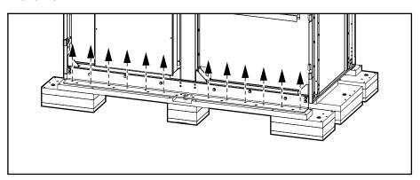
9. Install the jack bracket (TME58808) on the front transportation bracket with the four provided M8x30 bolts.
