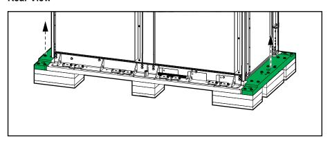
7. Remove the three floor protection plates (TME48195) and the jack (TME72611) from the cabinet. Save the three floor protection plates and the jack for later use.
