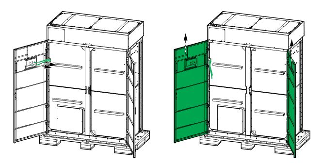
5. Remove the jack bracket (TME58808) from the right side of the pallet. Save the jack bracket for later use.
