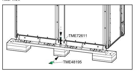
15. When the rear of the cabinet rests on the jack, remove the rear part of the wooden pallet from under the cabinet. Use a drilling machine or a wrench to turn the jack to lower the cabinet down onto the floor. Turn the jack until it can be removed from the rear transportation bracket.
