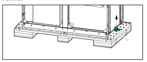
6. Remove the 16 wood screws and three long bolts from the left and right side of the pallet. Remove the left and right wooden parts.
