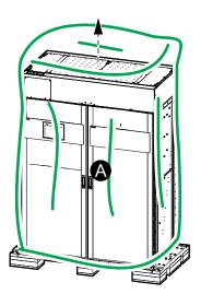
**NOTE:** Leave the four cardboard boxes on the rear of the I/O cabinet. These will be unpacked and used during installation.
