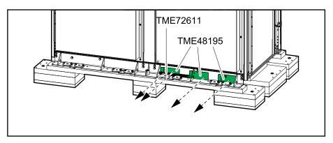
8. Remove the 12 wood screws from the front transportation bracket.
