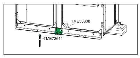
14. Place a floor protection plate (TME48195) under the rear part of the wooden pallet. Insert the jack (TME72611) in the rear transportation bracket. Use a drilling machine or a wrench to turn the jack to the right until the jack makes contact with the floor protection plate. Continue turning the jack to lift the cabinet.
