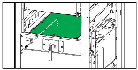
3. Install an additional AUX switch (provided) on the internal maintenance disconnect device IMB on both UPSs.
