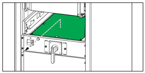
3. Remove the three single mains jumper busbars.
