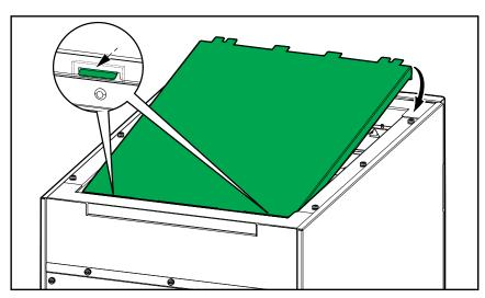
b. Push the top plate down in the front and reinstall the screws.
