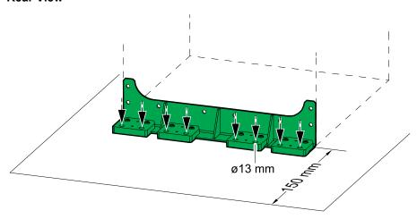
2. Remove the bolts and remove the rear anchoring bracket. Save the bolts for adjacent installation of cabinets.
