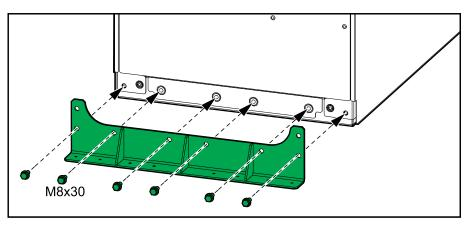
4. Push the UPS into position so the rear anchoring bracket connects to the rear anchors. The front anchoring bracket is installed in the final installation steps.
