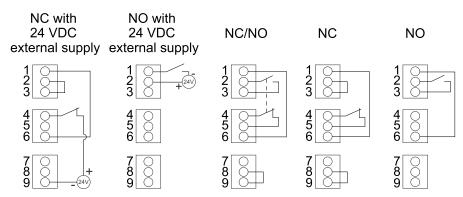
The EPO input supports 24 VDC.
