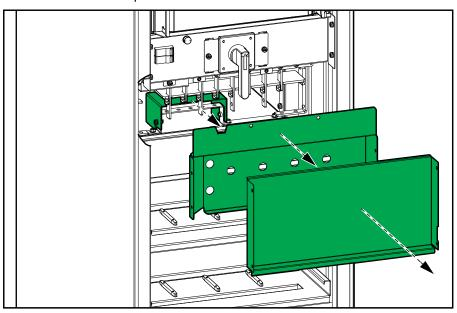
2. **Only for TN-C/3-wire earthing system**: Move the bonding busbar from position (A) to position (B) to connect the N busbar to the G/PE busbar.
