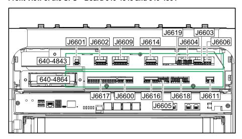
1. Connect the Class 2/SELV signal cables from the building EPO to board 640-4864 terminal J6600 in the UPS according to one of the options below.
