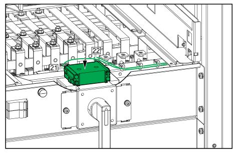
4. Connect the non-Class 2/non-SELV signal cables between the two UPSs.
