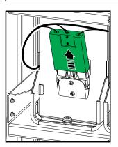
10. Remove the battery modules from the three upper rows. Leave the battery modules in the two bottom rows to increase weight stability.
