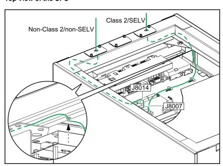
2. **Only for adjacent modular battery cabinet**: Route the provided signal cables 0W76627 and 0W12908 to board 640-7552 in the UPS.
