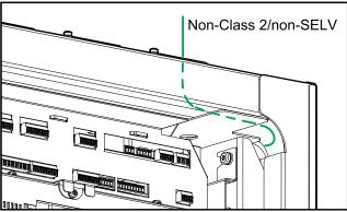
b. Route the Class 2/SELV cables and non-Class 2/non-SELV cables to board 640-7552 in the UPS.
