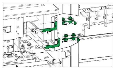
4. Connect the preinstalled DC cables from modular battery cabinet 1 to the DC extension busbars in the UPS.
