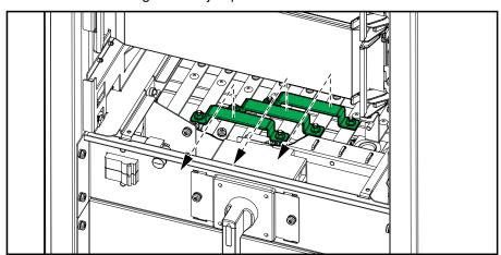
4. Reinstall the plate and the static switch module.
