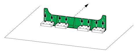
3. Install the rear anchoring bracket on the UPS with the provided M8 bolts.
