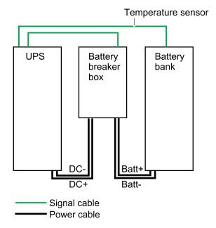
**NOTE:** Installation of the battery temperature sensor is not described in this manual, see the UPS installation manual for details.
