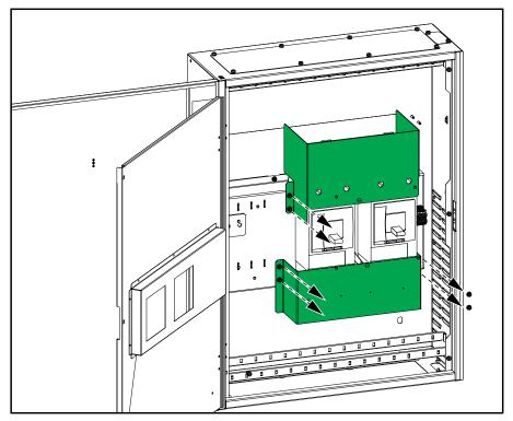
3. Route the signal cables through the top or bottom of the battery breaker box.
