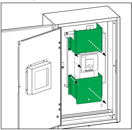
9. Measure for and verify ABSENCE of voltage on each DC busbar before continuing.
