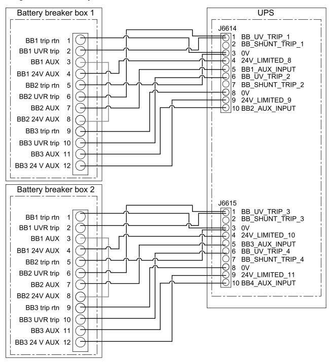
5. Route the signal cables separately from the power cables.
