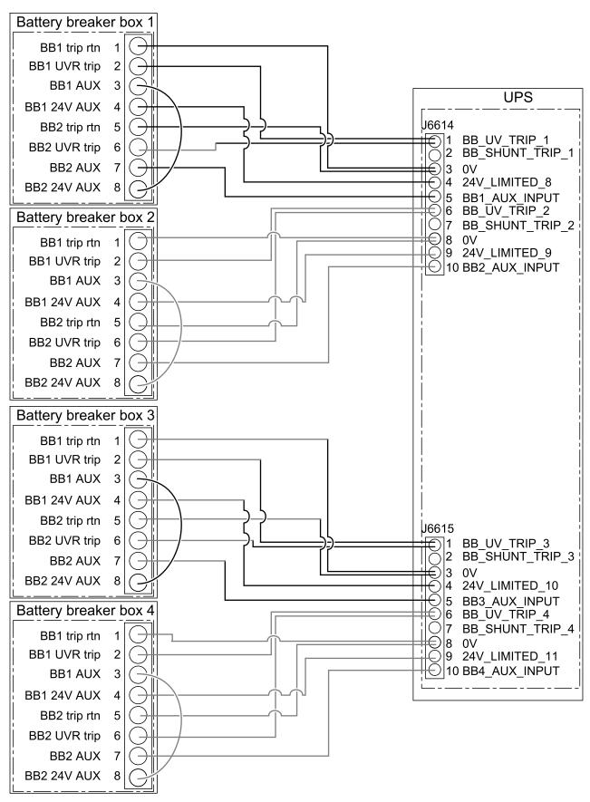
5. Route the signal cables separately from the power cables.
