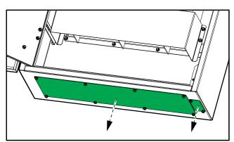
2. Drill or punch holes for power cables (A) and signal cables (B) or grommets in the gland plates, install grommets (if applicable), and reinstall the gland plates.
