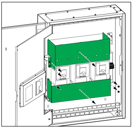
3. Route the signal cables through the top or bottom of the battery breaker box.
