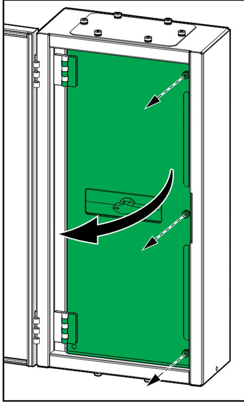
4. Mount the output switch box to the wall.
