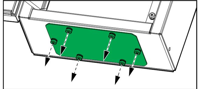
2. Drill or punch holes for cables or conduits in the gland plates.
