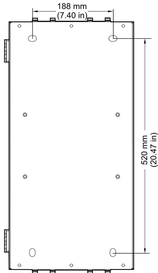
1. Measure and mark the four mounting hole locations on the wall.
