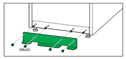
3. Push the UPS into position so the rear anchoring bracket connects to the rear anchor. The front anchoring bracket is installed in the final installation steps.
