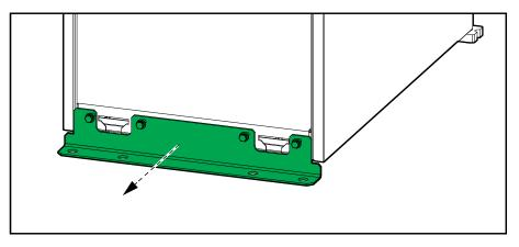
18. If the UPS is installed on the mounting skid kit GVSOPT027, dismount the UPS from the mounting skid. See the installation manual provided with the kit for details.
