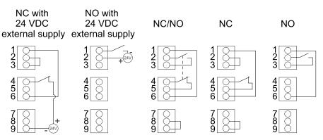
The EPO input supports 24 VDC.
