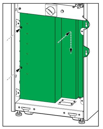
4. Reinstall the lower front plate.
