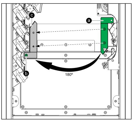
2. **Only for dual mains system**: Remove the three single mains jumper busbars.
