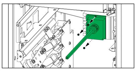
6. Install an additional AUX switch (provided) in the OF2 position in the internal maintenance disconnect device IMB on both UPSs.
