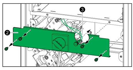
3. Disconnect the signal cables from the internal maintenance disconnect device IMB indicator light on both UPSs.
