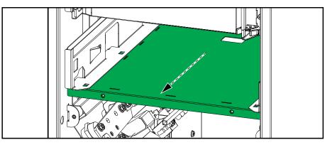
5. Remove the front cover from the internal maintenance disconnect device IMB on both UPSs.
