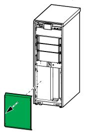
8. Measure for and verify ABSENCE of voltage with a multimeter probe through the holes in the transparent cover for input, bypass, output, neutral, and DC.
