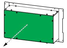
12. Measure for and verify ABSENCE of voltage on each input/bypass/output terminal before continuing.
