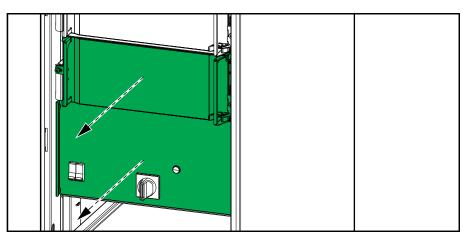
2. Install an additional AUX switch (provided) on the internal maintenance disconnect device IMB on both UPSs.
