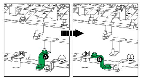
2. Remove the three single mains jumper busbars.
