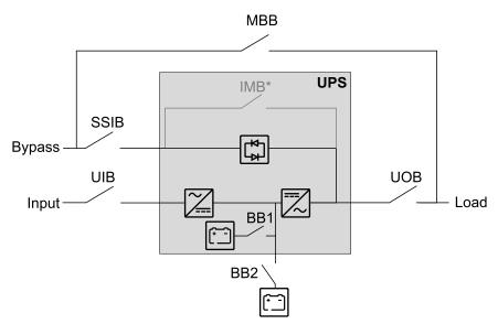
**NOTE:** IMB\* cannot be used in a system with an external MBB and IMB\* must be padlocked in the open position.
