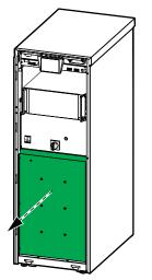
9. Disconnect the battery terminals from the front of all the battery modules.
