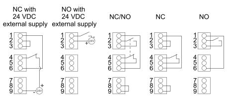
The EPO input supports 24 VDC.
