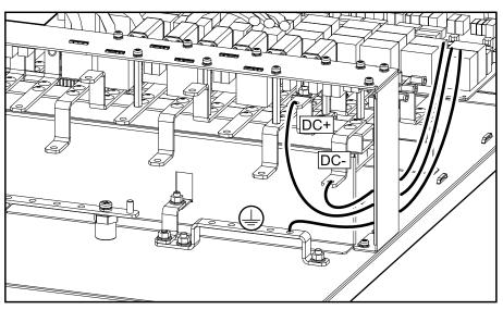
6. Route the equipment grounding conductor/PE cable and the DC cables into modular battery cabinet 1 and connect the equipment grounding conductor/ PE cable and DC cables in modular battery cabinet 1.
