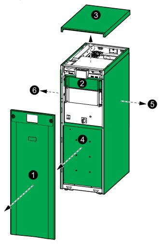
4. Remove the battery cover. Disconnect the battery terminals from the front of the battery modules.
