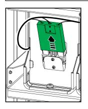
10. Remove the battery modules from the two upper rows. Leave the battery modules in the two bottom rows to increase weight stability.
