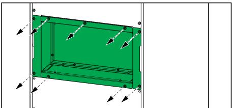
13. Remove the rear plate and the top or bottom gland plate from the conduit box.
