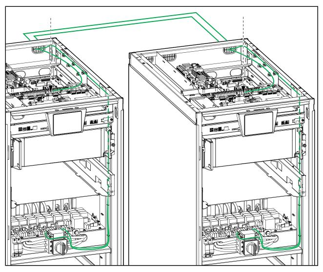
4. Reinstall the front cover and the static switch module on both UPSs.
