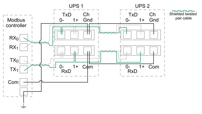
2. Install 150 Ohm termination resistors at each end of each bus if the buses are very long and operate at high data rates. Busses under 610 meters (2000 feet) at 9600 baud or under 305 meters (1000 feet) at 19200 baud should not require termination resistors.
