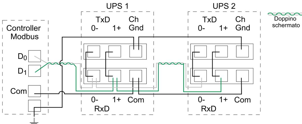
**Esempio: Connessione a 4 fili con 2 UPS**
