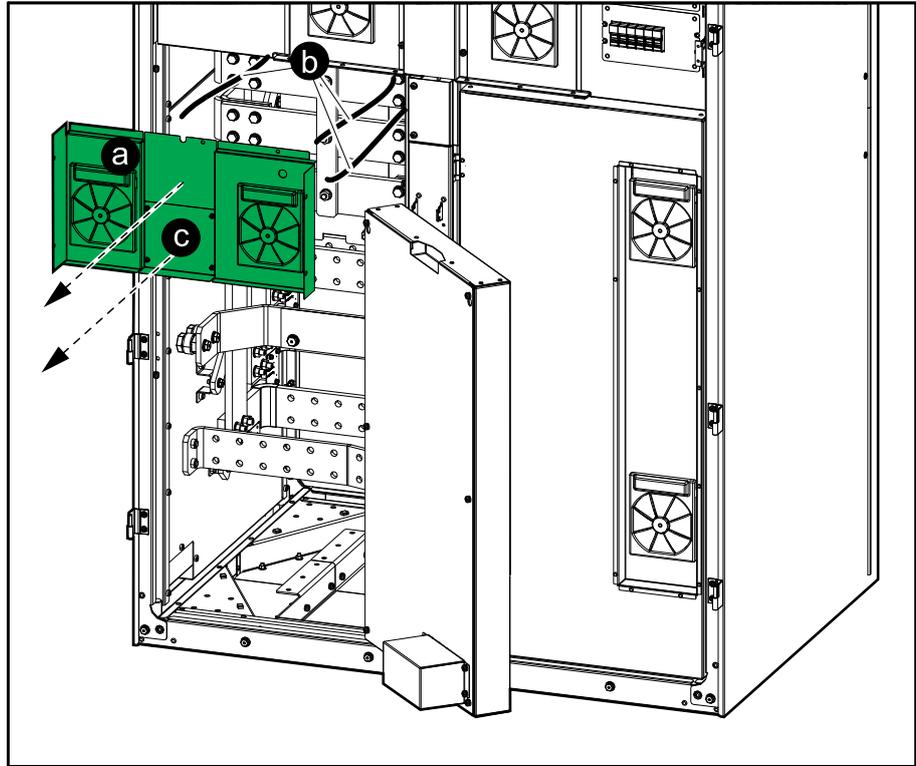
3. Remove the three busbars and the insulator part from the I/O cabinet.
