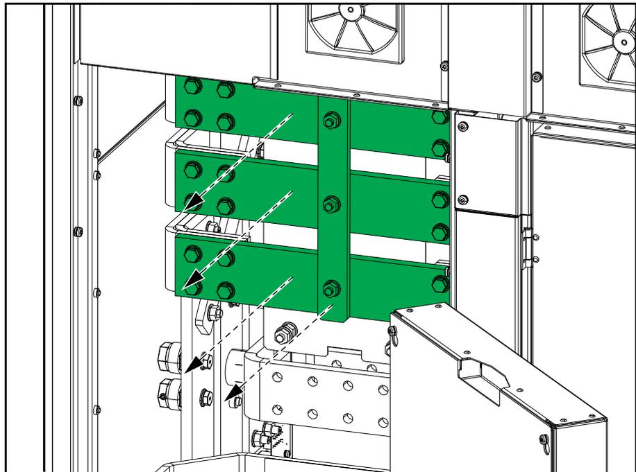
4. Remove the lexan plate from the I/O cabinet.
