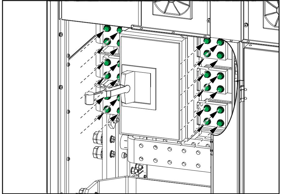
7. Install the signal cables in the backfeed breaker:
