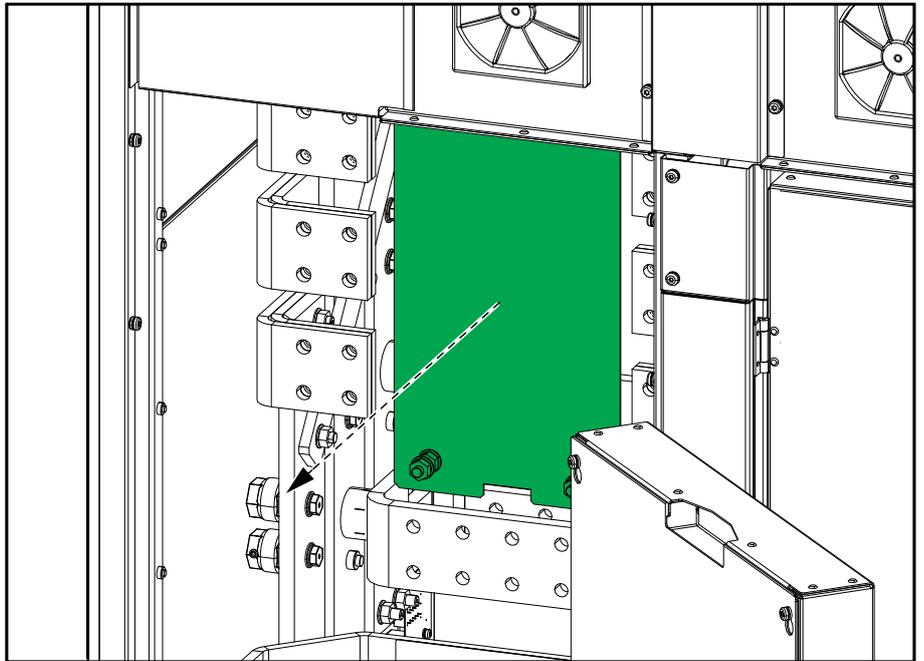
5. Install the backfeed breaker BF2 on the studs with the four provided nuts in the I/O cabinet.
