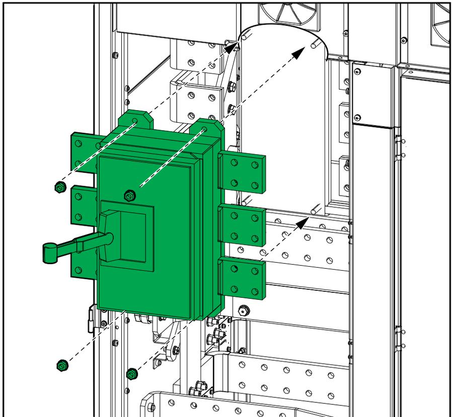
6. Connect the busbars to the backfeed breaker BF2 terminals. Reuse the 24 screws removed earlier.
