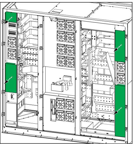
2. Remove the indicated plate for routing of non-Class 2/non-SELV cables.
