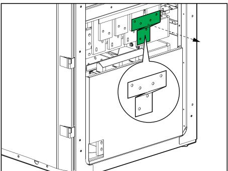
6. Remove and dispose of the indicated transport bracket from the right side of the I/O cabinet.
