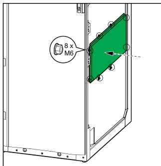
2. Install the interconnection cover 0M-82316 from the installation kit on the leftmost power cabinet.
