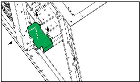
Remove the two gland plates from either the top or the bottom of the I/O cabinet and drill holes for the applicable Class 2/SELV and non-Class 2/non-SELV cables in the table below. Install conduits and reinstall the plates.
