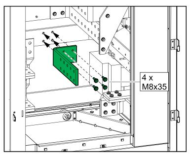
2. In installations with neutral connection only, remove the lexan plate from the N busbar.
