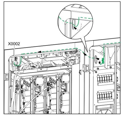
5. Route the signal cable connected in the right side of the I/O cabinet to the X0002 terminal in the power cabinet to the right of the I/O cabinet.
