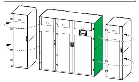
4. Remove and dispose of the indicated transport bracket from the left side of the I/O cabinet.
