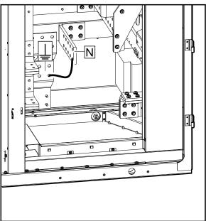
8. Only applicable to 4–wire systems: In an IT system, connect an external impedance between the N busbar and the earthing terminal.
