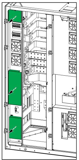
15. Remove the two indicated plates in the left side of the I/O cabinet.
