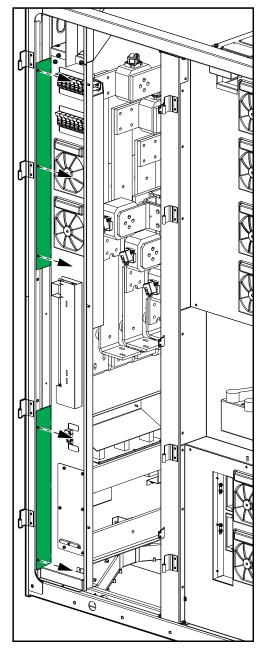
16. Mount the M6 screws from the installation kit from right to left in the four marked locations between the I/O cabinet and the power cabinet placed to the left of the I/O cabinet.
