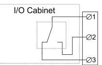
Output relay connection Max 5 A/250 VAC Max 5 A/24 VDC
