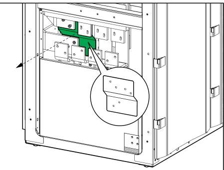
5. Remove and dispose of the indicated transport bracket from the right side of the I/O cabinet.
