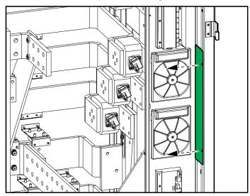
3. For bottom cable entry only: remove the plate in front of the cable channel for non-Class 2/non-SELV cables.
