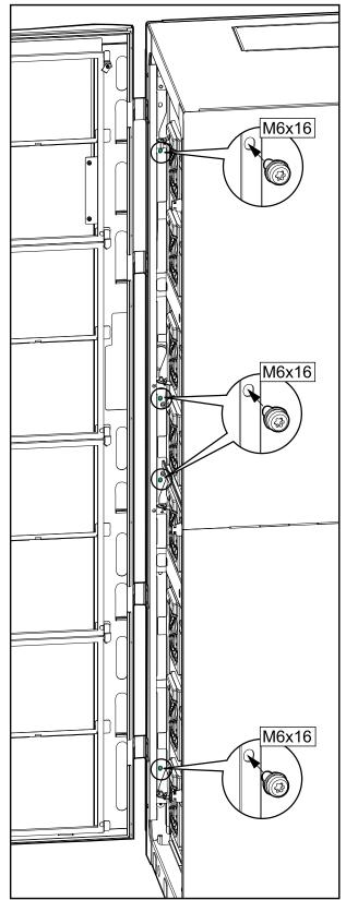
18. Verify that the right-most power cabinet and the left-most power cabinet for the I/O cabinet has the covers (0M-98993 and 0M-82316) and the side panels installed before continuing.
