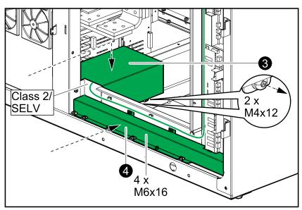
4. Reinstall the plate over the cable channel for non-Class 2/non-SELV cables.
