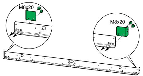
2. Place the rear anchoring brackets for the I/O cabinet and the power cabinets in the final installation area.
