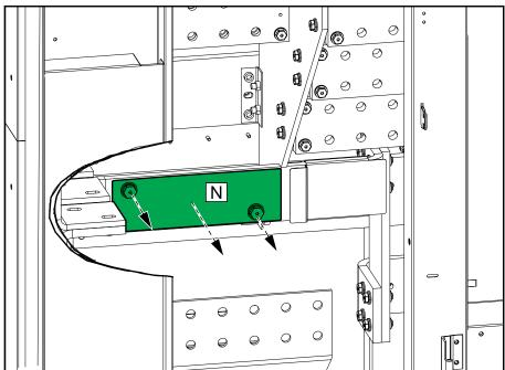
3. Connect the equipment earthing conductor/PE to the PE busbar.
