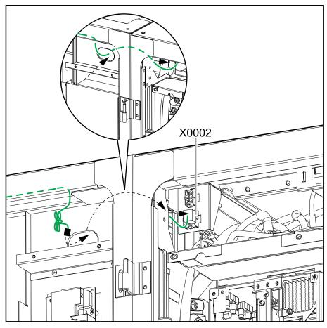
6. Route the signal cable 0W7819 from 0P6516 terminal J1005 in power cabinets 1–3 (on the left side of the I/O cabinet) and into the I/O cabinet as shown on the illustration and fasten the cable.
