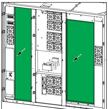
8. Push the I/O cabinet into position against the rear anchoring bracket – the I/O cabinet will connect to the conic outcroppings on the rear anchoring bracket.
