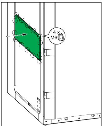
Remove the side panels from the I/O cabinet and install them on the left side of the left-most power cabinet and on the right side of the right-most power cabinet.
