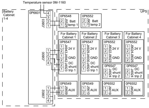
If the battery bank is consisting of two classic battery cabinets, connect signal cables between the two classic battery cabinets in one battery bank as shown.
