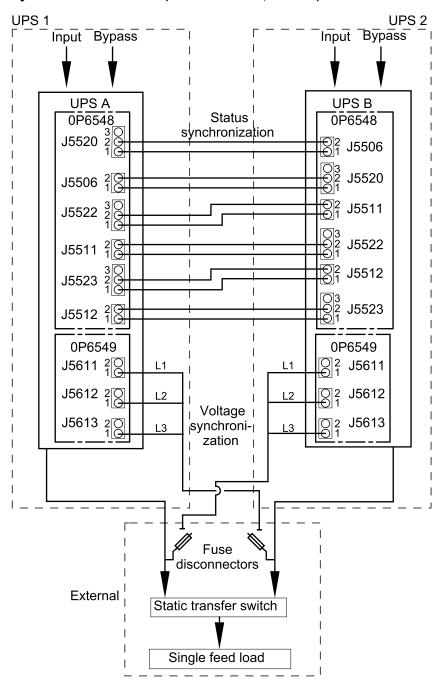
UPS with 1250 kW I/O Cabinet Signal Cables
