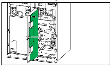
5. Close the door and fasten with the screw.
