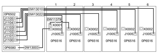
1. Remove the indicated plates from the I/O cabinet and all the power cabinets.
