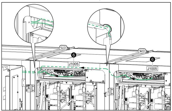
Signal Cables UPS with 1250 kW I/O Cabinet
