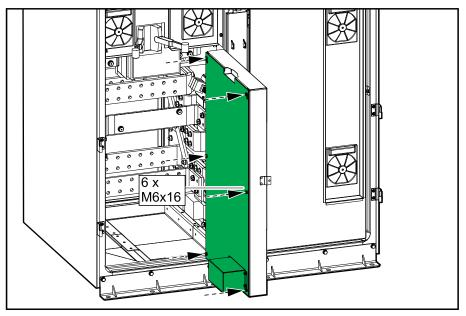
2. Close the door and fasten with the screw.
