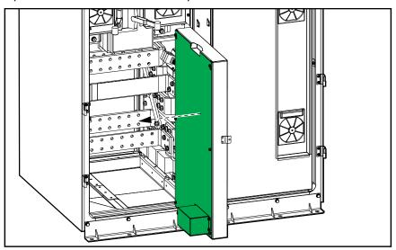
b. Route the external signal cables to the terminals and fasten with the provided cable ties.
