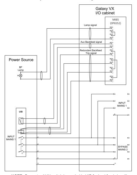
**NOTE:** One extra AUX switch is needed in UIB for backfeed signalling.
