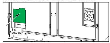
4. Reinstall the cover on the door in the right side and fasten with the screws.
