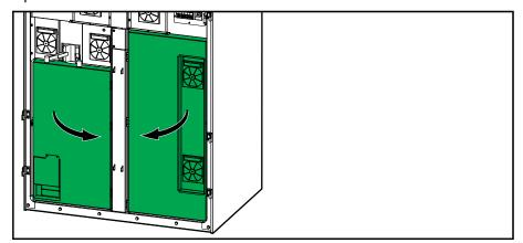
Measure for and verify ABSENCE of voltage on each input/bypass/output/DC busbar before continuing.
