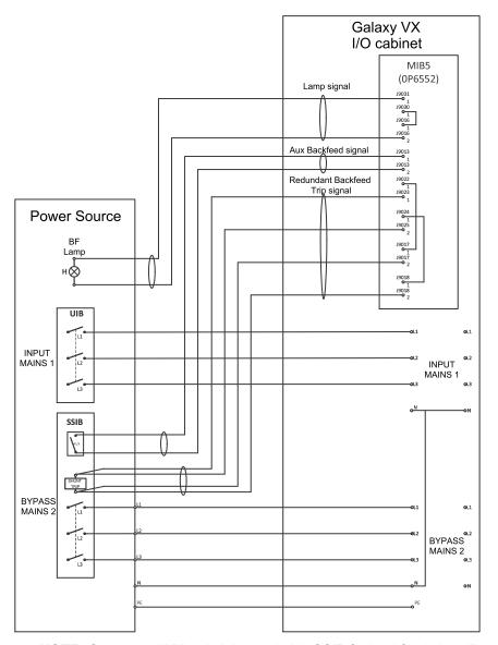
**NOTE:** One extra AUX switch is needed in SSIB for backfeed signalling.
