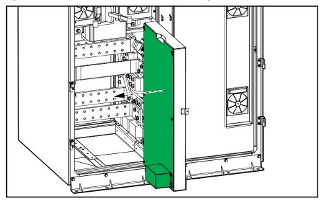
5. Route the signal cables 0W13022 (power cabinets 1-3) and 0W13010 (power cabinets 4-6) from the J1005 terminals in the power cabinets to the I/O cabinet.
