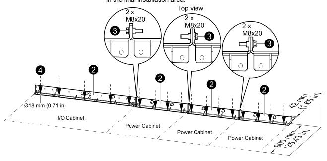
3. Interconnect the rear anchoring brackets using the provided screws and bolts.
