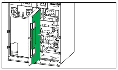
b. Route the cables to the board terminals and fasten with the provided cable ties. Class 2/SELV cables (A) must be routed separated from non-Class 2/non-SELV cables (B) as shown on the illustration.
