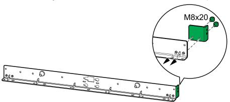
2. Place the rear anchoring brackets for the I/O cabinet and the power cabinets in the final installation area.
