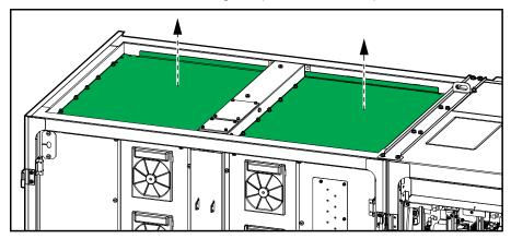
2. Drill or cut holes for cables/conduits in the top gland plate.
