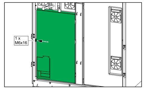
3. Reinstall the indicated cover if removed and fasten with the screws.
