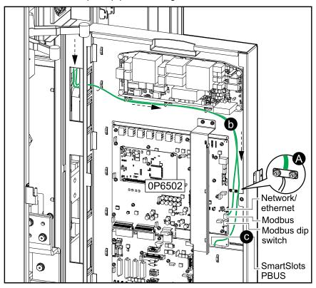
c. Close the door and route the PBUS cables and cables for the network management cards to the front.
