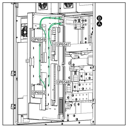
UPS with 1250 kW I/O Cabinet Signal Cables
