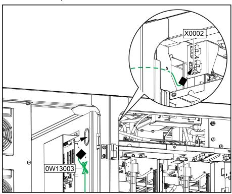
UPS with 1250 kW I/O Cabinet Signal Cables
