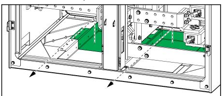
5. Push the I/O cabinet into position against the rear anchoring bracket - the I/O cabinet will connect to the conic outcroppings on the rear anchoring bracket.
