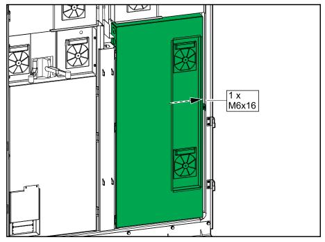
6. Reinstall the two indicated covers and close the door in the top right corner. Fasten with screws.
