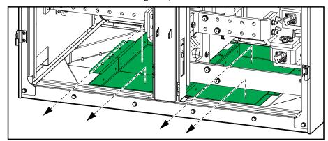
2. Drill or cut holes for cables/conduits in the bottom gland plate.
