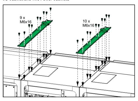
12. Mount the M6 screws from the installation kit from right to left in the five marked positions between the power cabinets and in the four marked positions between the power cabinet and the I/O cabinet to interconnect the cabinets.
