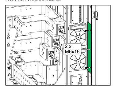
7. Reinstall the six plates in the left and right sides of the I/O cabinet.
