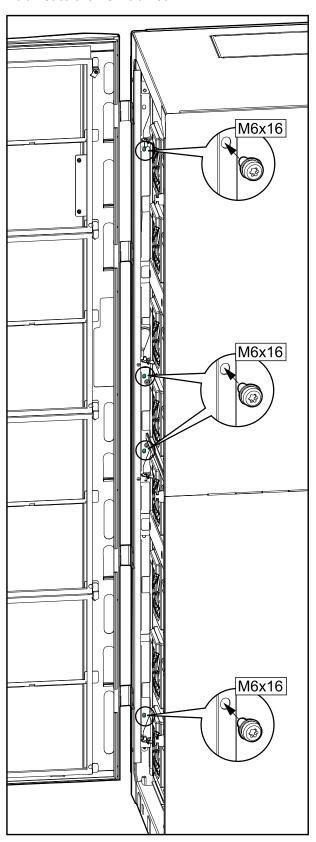
18. Verify that the right-most power cabinet and the left-most power cabinet for the I/O cabinet has the covers (0M-98993 and 0M-82316) and the side panels installed before continuing.
