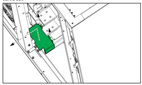
6. Remove the two gland plates from either the top or the bottom of the I/O cabinet and drill holes for the applicable Class 2/SELV and non-Class 2/non-SELV cables in the table below. Install conduits and reinstall the plates.
