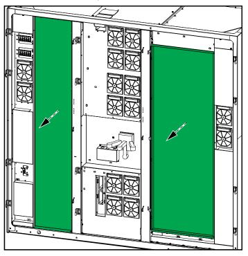
8. Push the I/O cabinet into position against the rear anchoring bracket – the I/O cabinet will connect to the conic outcroppings on the rear anchoring bracket.
