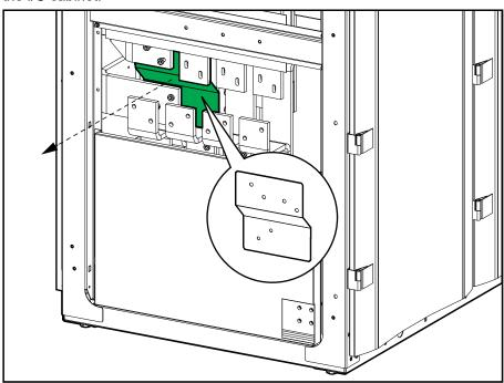
5. Remove and dispose of the indicated transport bracket from the right side of the I/O cabinet.
