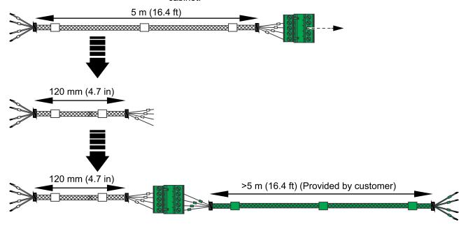
Select the extension signal cables according to the Signal cable specifications.
