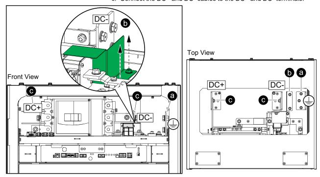
Connect the power cables in the UPS. If more battery cabinets are part of the solution, connect all battery cabinets to the UPS according to the diagram below.
