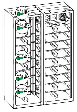
6. Push the third battery cabinet into position, align with the seismic anchoring (if any), level the battery cabinet, and interconnect with the other battery cabinets as described in step 2, step 3, and step 5. Continue until all the battery cabinets are in place, levelled, and interconnected.
