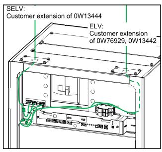
5. Route the signal cable 0W76928, 0W76934, and 0W76972 through the openings in the sides of the battery cabinets and to the ports in the rack BMS and the switchgear ports. Do not connect the signal cables, Schneider Electric service will complete the connections during start-up.
