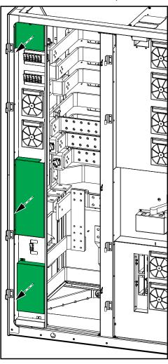
15. Remove the two indicated plates in the left side of the I/O cabinet.
