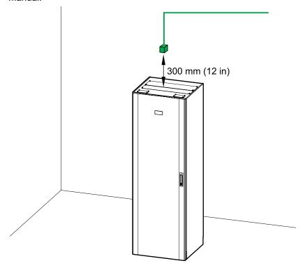
**NOTE:** The temperature sensor measures the ambient temperature. Do not place the temperature sensor close to external heating or cooling equipment which may give an incorrect measurement of the ambient temperature.
