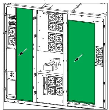
8. Measure for and verify ABSENCE of voltage on each input/bypass/output/DC busbar before continuing.
