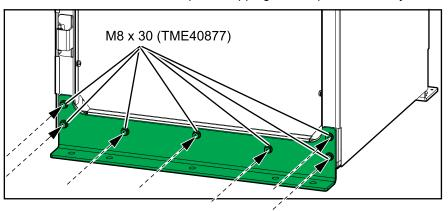
2. Anchor the front seismic bracket to the floor using appropriate hardware for the floor type – the hole diameter in the front seismic bracket is ø14 mm. The minimum requirement is M12 strength grade 8.8 hardware.
