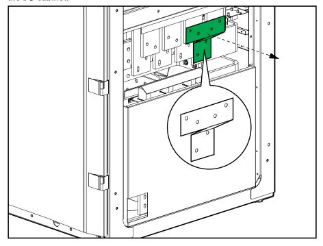
6. Remove and dispose of the indicated transport bracket from the right side of the I/O cabinet.
