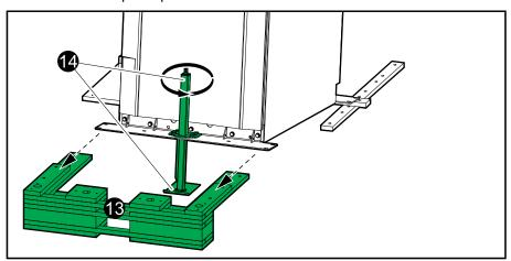
14. Use the jack to lower the cabinet onto the floor until the wheels connect with the floor. Remove the jack and the floor protection plate.
