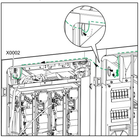
5. Route the signal cable connected in the right side of the I/O cabinet to the X0002 terminal in the power cabinet to the right of the I/O cabinet.
