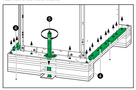
5. Use a drilling machine with the provided hexagonal socket to activate the jack, slide it into position in the bracket, and to make contact with the floor protection plate.
