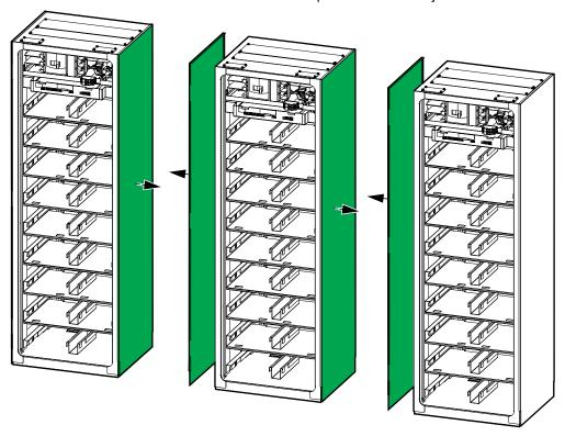
2. Push the right-most battery cabinet into position. For seismic anchoring, ensure that the rear seismic bracket connects to the rear anchors.
