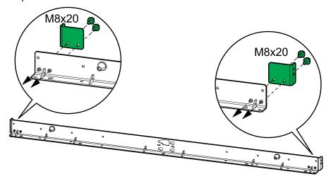
2. Place the rear anchoring brackets for the I/O cabinet and the power cabinets in the final installation area.
