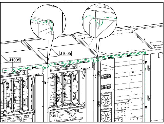
7. Route the signal cable 0W7822 from 0P6516 terminal J1005 in power cabinet 4 and power cabinets 5–6 if available (on the right side of the I/O cabinet) and into the I/O cabinet as shown on the illustration and fasten the cable.
