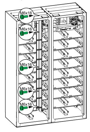
6. Push the third battery cabinet into position, align with the seismic anchoring (if any), level the battery cabinet, and interconnect with the other battery cabinets as described in step 2, step 3, and step 5. Continue until all the battery cabinets are in place, levelled, and interconnected.
