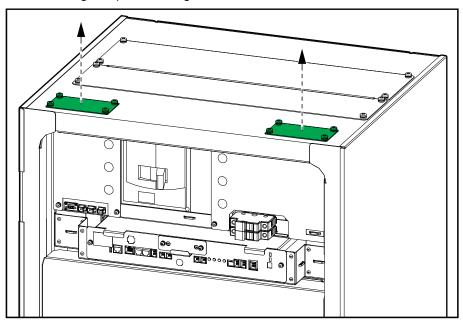
2. Drill or punch holes for cables/conduits and install conduits (if applicable).
