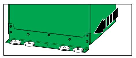
3. Lower the levelling feet until they connect with the floor - use a bubble-leveler to ensure that the cabinet is level.
