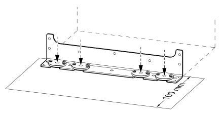
9. In systems with more battery cabinets, interconnect the seismic assemblies with the interconnection plate 870-51172 from the accessory kit 0M-95331.
