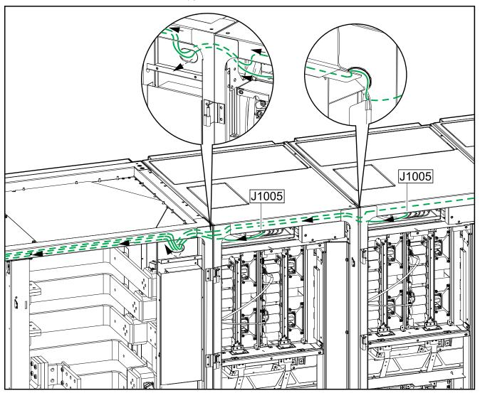
8. In redundant systems only, route the signal cable 0W7827 from 0P6516 terminal J1005 in power cabinet 7 and into the I/O cabinet and fasten the cable.
