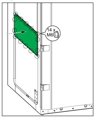
3. Remove the side panels from the I/O cabinet and install them on the left side of the left-most power cabinet and on the right side of the right-most power cabinet.
