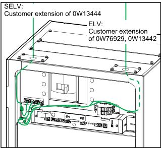
5. Route the signal cable 0W76928, 0W76934, and 0W76972 through the openings in the sides of the battery cabinets and to the ports in the rack BMS and the switchgear ports. Do not connect the signal cables, Schneider Electric service will complete the connections during start-up.
