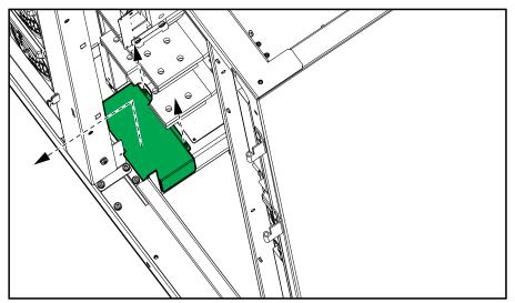
6. Remove the two gland plates from either the top or the bottom of the I/O cabinet and drill holes for the applicable Class 2/SELV and non-Class 2/non-SELV cables in the table below. Install conduits and reinstall the plates.
