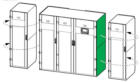
4. Remove and dispose of the indicated transport bracket from the left side of the I/O cabinet.
