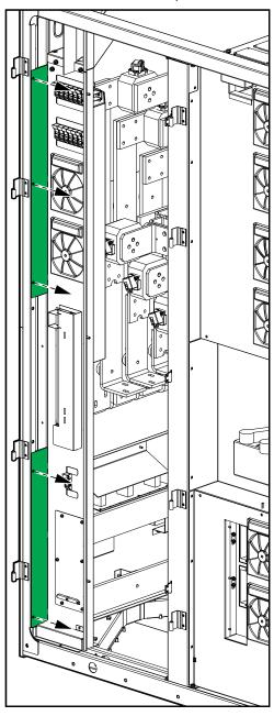
16. Mount the M6 screws from the installation kit from right to left in the four marked locations between the I/O cabinet and the power cabinet placed to the left of the I/O cabinet.
