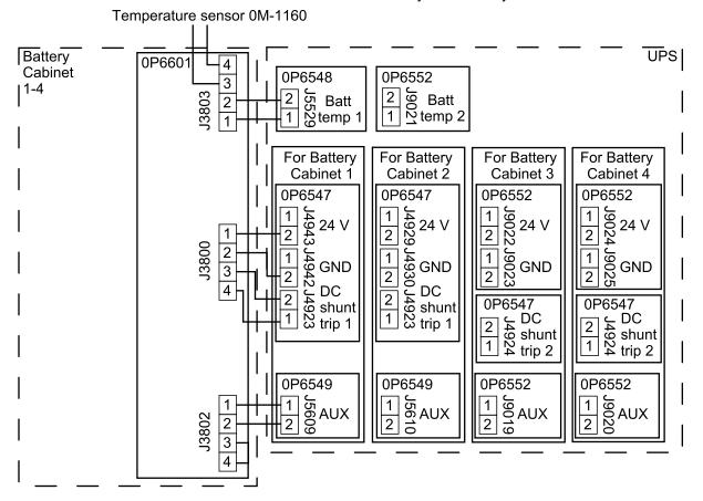
If the battery bank is consisting of two classic battery cabinets, connect signal cables between the two classic battery cabinets in one battery bank as shown.
