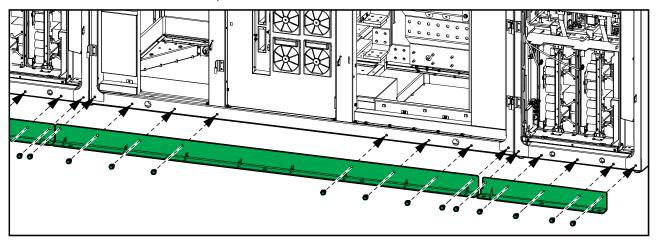
2. Anchor the front anchoring brackets to the floor.
