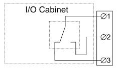
Output relay connection Max 5 A/250 VAC Max 5 A/24 VDC
