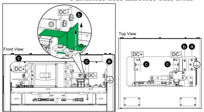
5. Connect the power cables in the UPS. If more battery cabinets are part of the solution, connect all battery cabinets to the UPS according to the diagram below.
