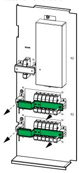
3. Click the AUX switch onto the left side of the battery control breakers. Click the two battery control breakers with AUX switches onto the DIN rails.
