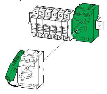
4. Tighten or reinstall the DIN rails.
