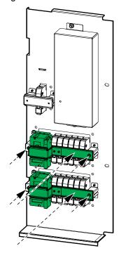
5. Disconnect the ten cables from the terminal block.
