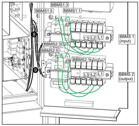
Close the upper right inner door and fasten with the screws. Install the new covers (870-65262), reuse the screws from step 1 and torque to 5 Nm (3.69 lb-ft / 44.3 lb-in).
