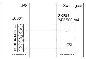
**NOTE:** SKRU presence must be configured by Schneider Electric Service at start-up.
