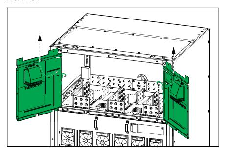
2. **Only for dual mains system**: Remove the three single mains busbars. Save the three single mains busbars for testing during start-up of the UPS.
