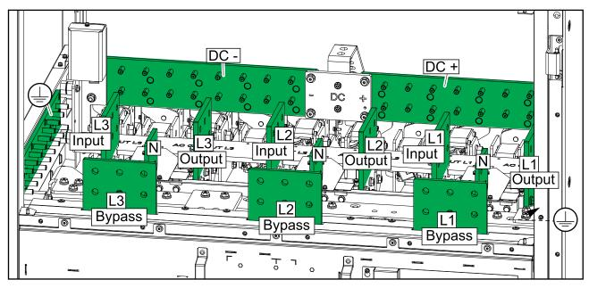
11. Disconnect all power cables from the UPS. See Connect the Power Cables in the UPS, page 72 for details.
