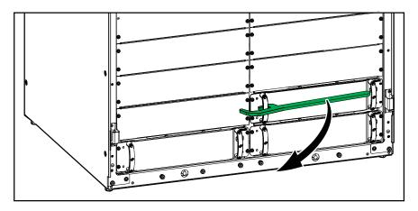
Front View of Using the Power Module Tool When the Power Module is Next to an Empty Slot
