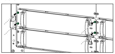
4. Set the enable switch on the power module to the ON (locked) position.
