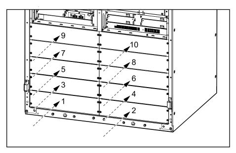
1. Remove the filler plate from the empty power module slot. Save the filler plate for future use. Save the screws for reuse.
