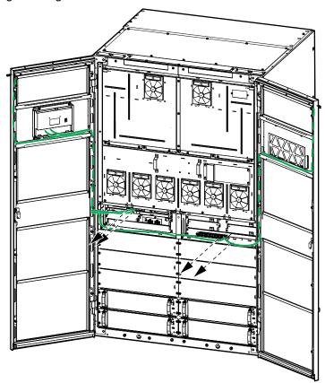
4. Remove kit 0M-18450 (bag with spring washers) from the documentation compartment in the right front door and save for later use.
