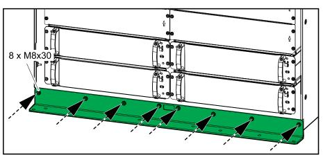
17. Mount the front seismic anchoring bracket to the floor. Use appropriate hardware for the floor type – the hole diameter in the front seismic anchoring bracket is ø16 mm. Minimum requirement is M12 strength grade 8.8 hardware (not provided).
