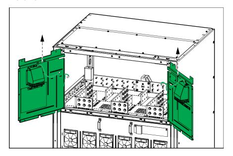
Remove the transparent protection cover from the external synchronization board 0P4809. Connect the cables for external synchronization to the external synchronization board 0P4809.
