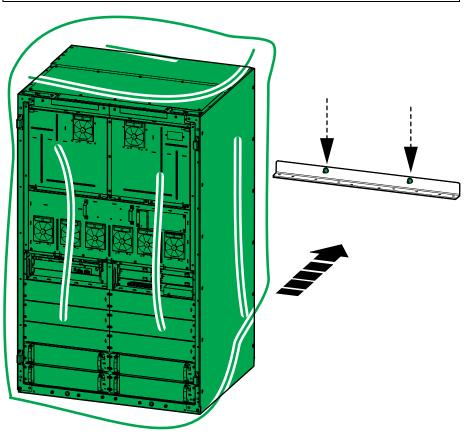
8. Fasten the cabinet to the rear seismic anchoring bracket by tightening the bolts. Torque to 50 Nm (36.87 lb-ft).
