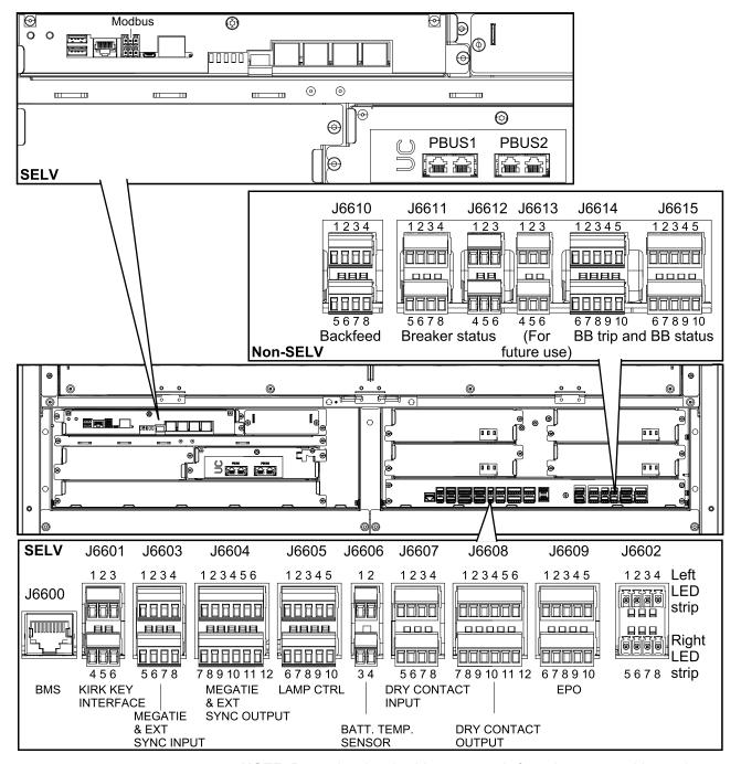
**NOTE:** Route the signal cables separately from the power cables and route the Class 2/SELV cables separately from the non-Class 2/non-SELV cables.
