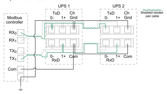
2. Install 150 Ohm termination resistors at each end of each bus if the buses are very long and operate at high data rates. Busses under 610 meters at 9600 baud or under 305 meters at 19200 baud should not require termination resistors.
