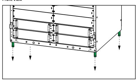
**NOTE:** For installations with limited rear access, only lower the two front feet.
