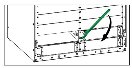
Front View of Using the Power Module Tool When the Power Module is Next to a Power Module
