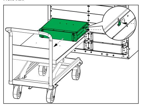
e. Install a filler plate in front of the empty power module slot, if available.
