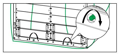
9. Lower the two front feet on the UPS until they have full contact with the floor – use a bubble-leveler to ensure that the cabinet is level.
