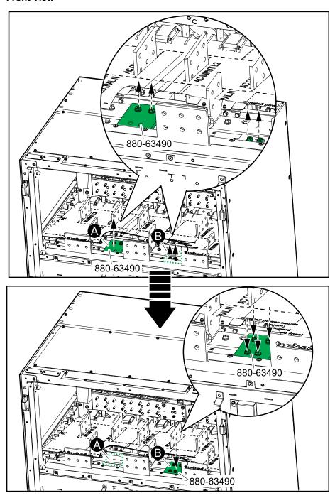
4. Connect the power cables in the described order. Assemble the cable lugs to the busbars as shown.
