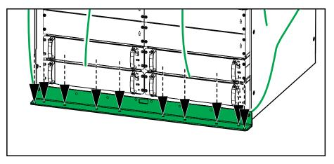
13. Remove the front anchoring bracket from the UPS. Secure the packaging bag against the UPS with tape to create a seal.
