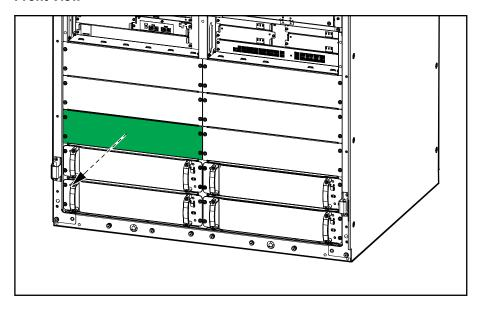
2. Use an appropriate scissor lifting cart to lift the power module to the correct height and push the power module into the power module slot.
