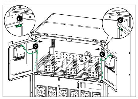
e. Lift the inner doors upwards to remove them.
