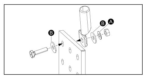
Spring washer (A) – provided in kit 0M-18450. Flat washer (B) (not provided).
