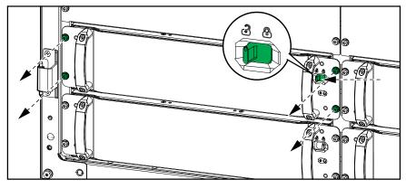
Use the provided power module tool to pull the power module out from the power module slot. Place the tool as shown.
