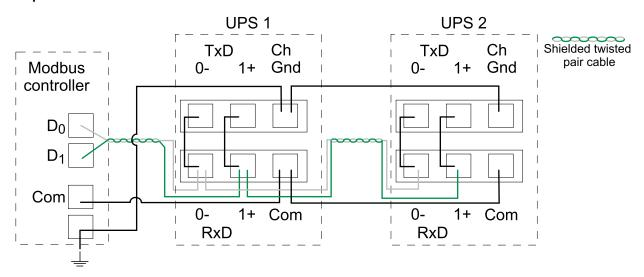
UPS Connect the Modbus Cables
