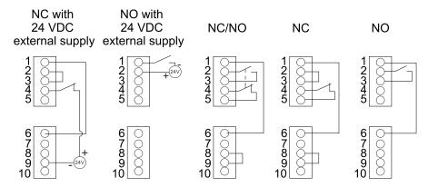
The EPO input supports 24 VDC.
