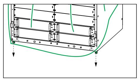
10. Remove the eight M8x30 screws from the front of the UPS. These screws are needed for the front seismic anchoring bracket.
