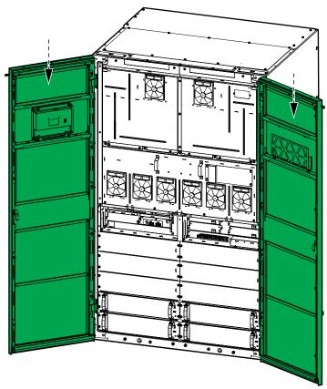
Reconnect the display signal cable and the two LED strip signal cables to the cabinet.
