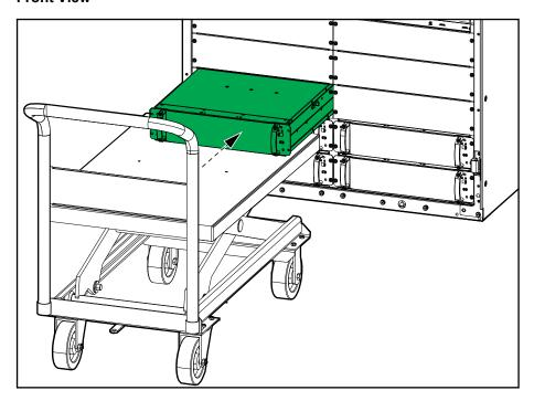
3. Install the four screws in the left and right sides of the power module. Reuse the screws from step 1.
