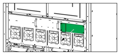
7. Measure for and verify ABSENCE of voltage with a multimeter probe through the holes in the transparent plate for input, bypass, output, neutral, and DC.
