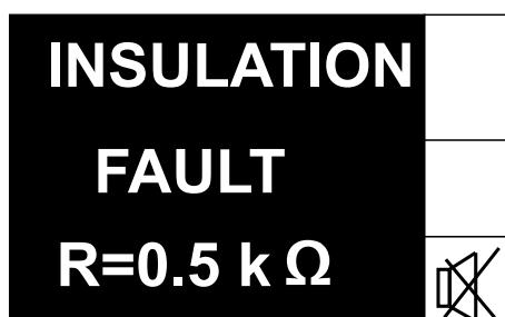
The screen flashes whenever an insulation alarm is detected.
