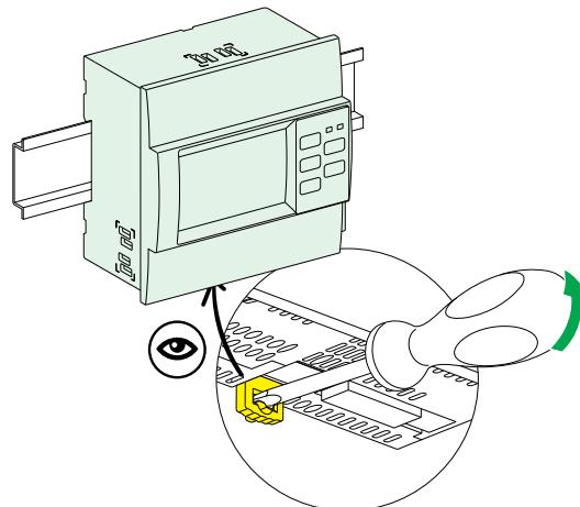
3. Lift the device up to free it from the DIN rail.
