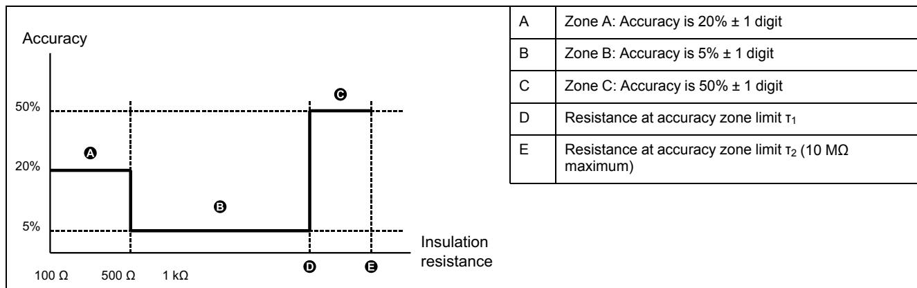
Assuming two significant digits for insulation resistance measurements the accuracy can be calculated.
