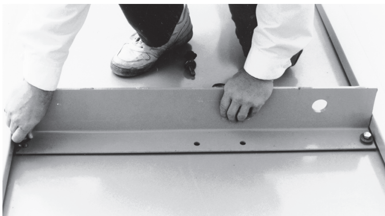
Figure 10 - Removing Small Lifting Lugs
