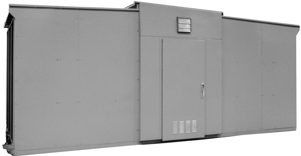
The common aisle switchgear is shipped with the “low side” and the “high side” switchgear sections fully assembled and ready to set on a concrete pad. The aisle is shipped in subassemblies.
