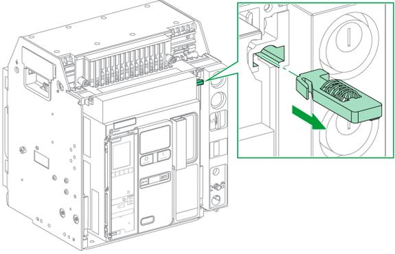
The diagram shows a side view of the circuit breaker cabinet with the handle door open. A green callout box provides a magnified view of the interlocking button being pulled out from its slot. A green arrow indicates the direction of removal. |
