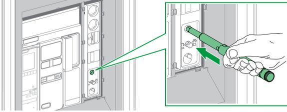
The diagram shows the handle door open. A green callout box shows a hand inserting a green handle into the slot. A green arrow indicates the insertion direction.                                                                                  |
