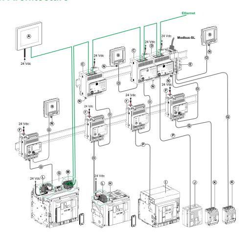
A FDM128 Ethernet display for eight devices
