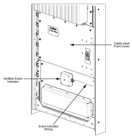
Figure 82 - Cable Vault Front Cover Labels
