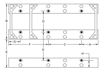
● = Seismic Tie-Down Locations
