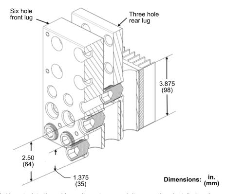
Figure 75 - Lug Cross Section Showing Hole Placement
