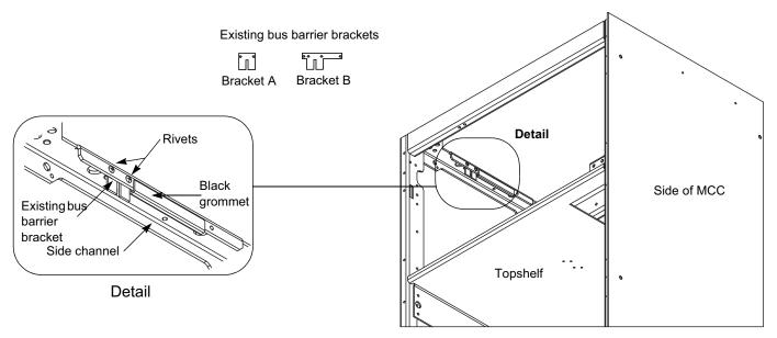
**NOTE:** Discard all retrofit brackets if the existing bus barrier bracket "B" (see Remove Existing Brackets on the 15 in. (381 mm) Deep MCC, page 215) is present on the 15 in. (381 mm) deep MCC. All holes are already present for direct mounting of the horizontal bus barrier.
