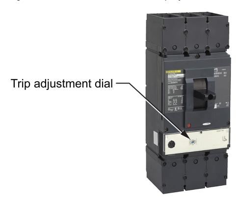
After obtaining the motor full load current from the motor nameplate, select an adjustable trip set-point to test start the motor. Further adjustments may be required because of motor load characteristics. Refer to applicable national installation codes for permissible set-points.
