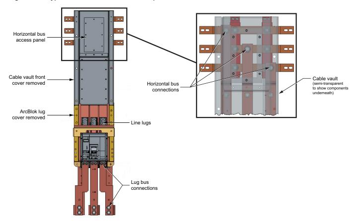
7. Verify that all main lug, circuit breaker, or fusible switch set screws holding incoming conductors in main lugs are in place and properly tightened (see Main Lug Compartment Torque Connection, page 119). Use a torque wrench and a 3/8 in. Allen bit to torque the lug set screws to the appropriate value (see Cable Connection Torque Values, page 110).
