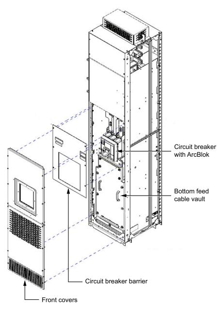
Figure 70 - Line-side Isolation Cable Vault and ArcBlok Bottom-feed Main Lug Breaker Access
