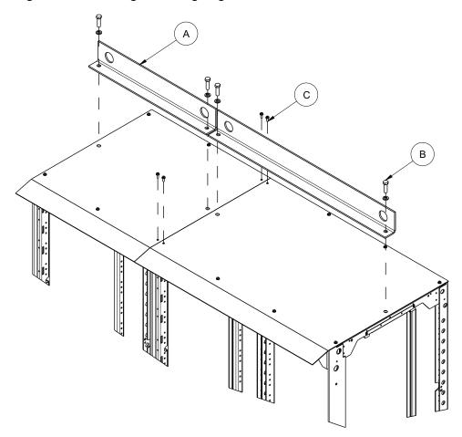
2. Uninstall and discard the lifting angles (A) by removing the 3/8-in bolts and washers (B) securing them.
