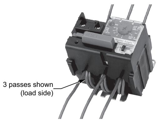
Passes begin from the load side of the overload through the CT window and return via the windows provided between the baseplate and overload (see MotorLogic Overload (Bottom View), page 145). The final pass terminates on the load side of the contactor.
