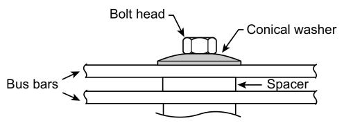
Torque the splice connection bolts at horizontal bus connections to 31–32 lb-ft. (41.87–43.22 N•m). Torque 85 kA support nuts (if applicable) to 68–72 lb-ft. (92.2–97.6 N•m) (see Torque All Bolts, page 66).
