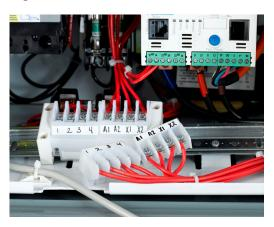
Figure 169 - Connecting Control Leads to the Terminal Blocks
