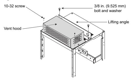
3. Remove the two 10-32 screws that secure the vent hood and closing plate to the top of the cabinet (see Reposition and Attach the Vent Hood, page 98).
