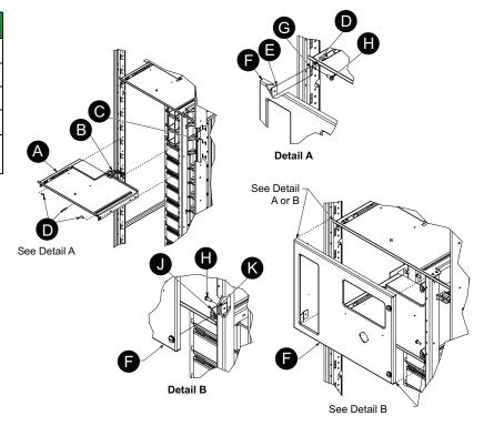
Figure 195 - Automatic Vertical Bus Shutter Installation—Style 2
