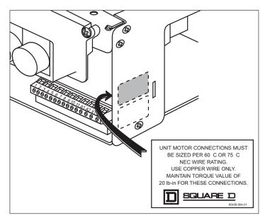
**NOTE**: Removal of the control station plate may be necessary to install power and control wiring. For detailed steps, refer to step 4 in Removing the Compac<sup>™</sup> 6 Control Unit, page 127.
