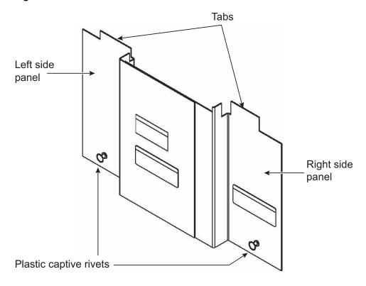
Figure 177 - Horizontal Bus Barrier Installation and Removal
