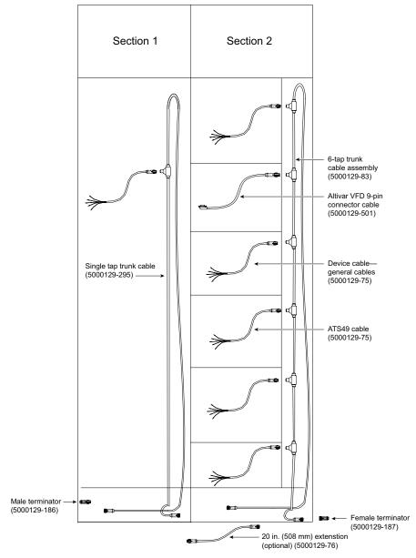
Figure 153 - Typical Cabling Scheme for DeviceNet and CANopen (8A cable)
