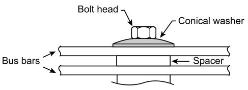
6. Torque all bolts on both ends to 31–32 lb-ft. (41.87–43.22 N•m) (see Torque All Bolts, page 69).
