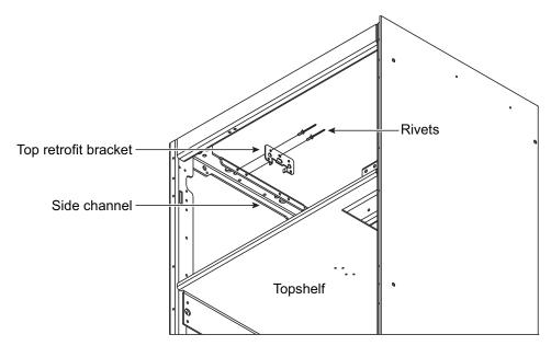
20 in. (508 mm) deep MCC: Use the screws provided in the retrofit kit to attach
