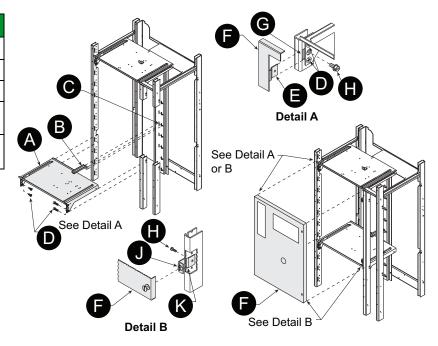
Figure 192 - Automatic Vertical Bus Shutter Installation—Style 1
