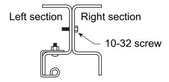
9. If the lifting angle is to be removed from the sections after installation, replace all hardware in the order shown (see Replace Lifting Angle Hardware, page 56).
