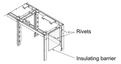
6. Install the deflector bracket (see Installing the Deflector Bracket, page 50) on the right most section of the MCC being added using two 8-32 Phillips head screws included in the kit. The same holes from which the rivets were removed are used to mount the deflector bracket. The top holes of the bracket must align with the holes in the top plate of the enclosure.
