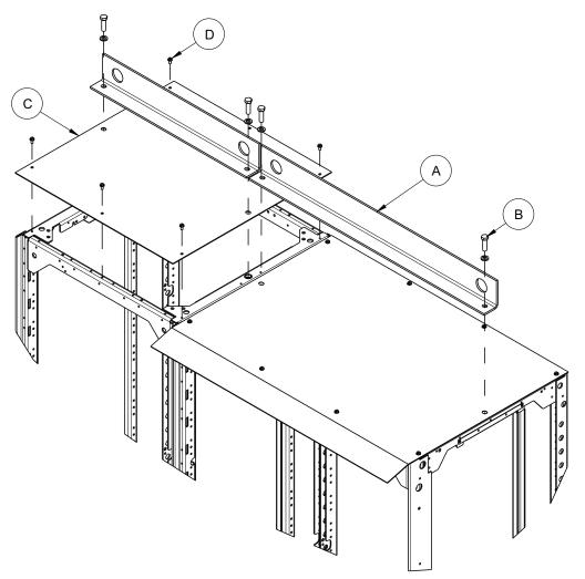
1. Uninstall and discard the lifting angles (A) by removing the 3/8 in. bolts and washers (B) securing them.
