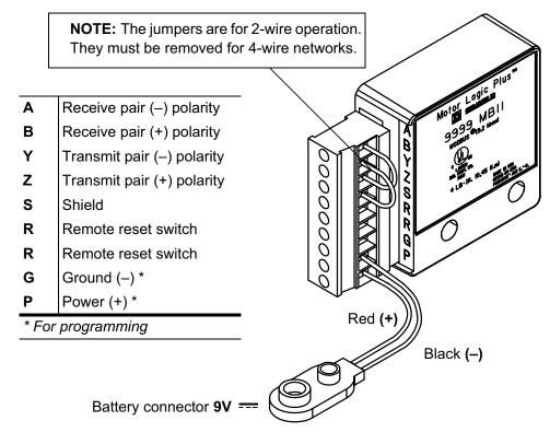
4. Turn the "Mode Select" switch to the parameter you are programming. Refer to Schneider Electric instruction bulletin 30072-013-98 (see iMCC-related Literature, page 17) for a list of parameters.
