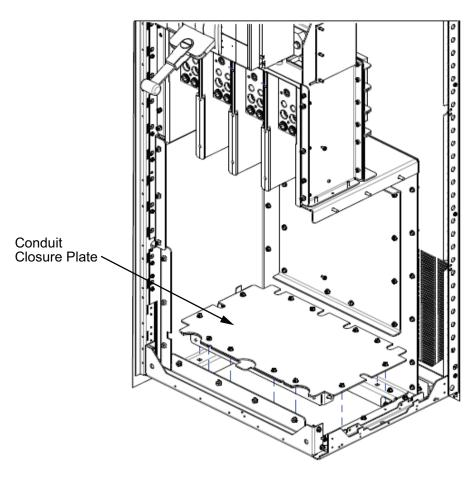
8. Pull the cables inside the cable vault and terminate them on the ArcBlok lugs shown in Lug Cross Section Showing Hole Placement, page 84. Torque all wire-binding screws to 842 lb—in. (95 N•m).
