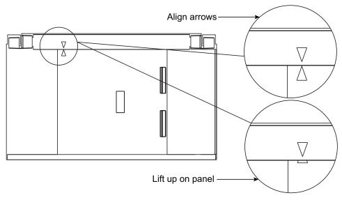
3. Align the arrows on the right panel and top track as shown in Installing the Right Panel into the Rear Groove, page 220. Lift the panel out of the bottom track and remove the panel.
