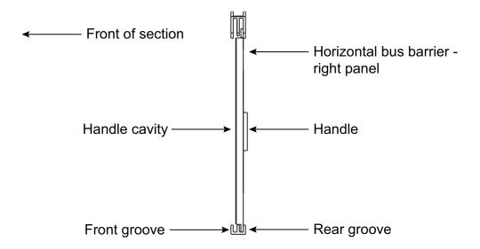
1. Align the arrows on the right panel and top track as shown in Installing the Right Panel into the Rear Groove, page 220.
