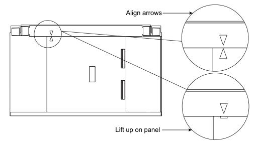
4. Align the arrows on the right panel and top track as shown in Aligning the Arrows on the Panels, page 208. Lift the panel out of the bottom track and remove the panel.
