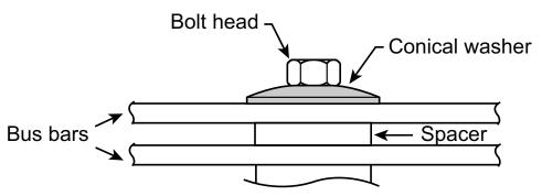
4. Torque all bolts on both ends to 31–32 lb-ft. (41.87–43.22 N•m). (See Torquing the Bolts, page 61).
