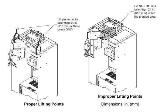
Before installing any MCC control units, locate and retighten or re-torque any connections that may have loosened during shipment and handling. Refer to the procedures in Installing Additional MCC Units, page 181.
