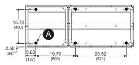
A Structure anchoring locations (typical of 4)
