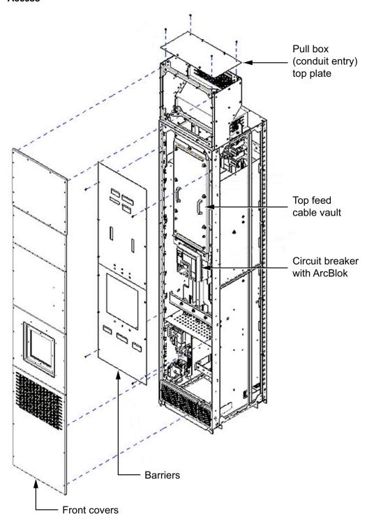
Figure 68 - Line-side Isolation Cable Vault and ArcBlok Top-feed Main Lug Breaker Access
