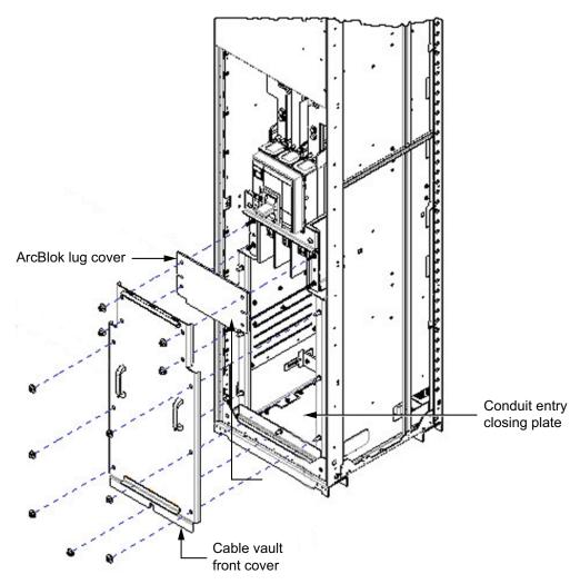
**NOTE:** Cable entry into line-side isolation cable vaults must use conduit connection means installed on the closing plate (in bottom-feed applications) or the pull box top closing plate (in top-feed applications). Conduits must be sealed using duct seal putty.
