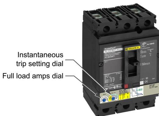
Figure 128 - PowerPacT H- and J-frame Magnetic Trip Adjustment
