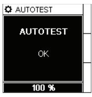
• If the auto test fails, the **Product Status** LED turns ON and a message is displayed to indicate that the product is malfunctioning. Disconnect the auxiliary power supply of device and reconnect. If the fault persists, contact technical support.
