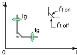
The ground-fault protection threshold  $I_g$  sets the level of ground-fault current at which the circuit breaker trips when reaching the ground-fault protection time delay  $t_g$ .
