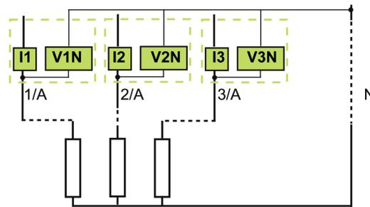
When there is voltage measurement on the neutral (4-pole or 3-pole circuit breaker with ENVT wired and configured), the control unit measures the power by using 3 single-phase loads downstream.
