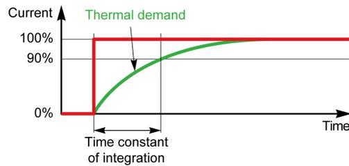
The time constant of integration (current demand calculation interval) is fixed and set at 15 minutes.
