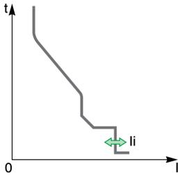
Instantaneous overcurrent protection for MicroLogic Active 5.0 and 6.0 can be enabled or disabled with EcoStruxure Power Commission software.
