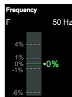
Green color indicates measurement is OK: the difference between the measured and expected frequency is less than 1%
