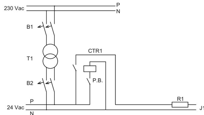
Use 2.5 mm<sup>2</sup> cables between R1 and CTR1.
