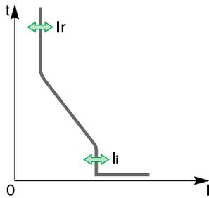
The instantaneous overcurrent protection setting is  $I_i$ : instantaneous overcurrent protection threshold (corresponds to a short-time overcurrent protection threshold without time setting).
