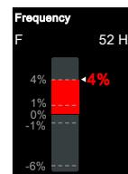
Red color indicates measurement is significantly out of range: the difference between the measured and expected frequency is greater than +4% or less than -6%
