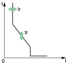
Long-time overcurrent protection is based on the true RMS current of phases and neutral, up to harmonic 15.
