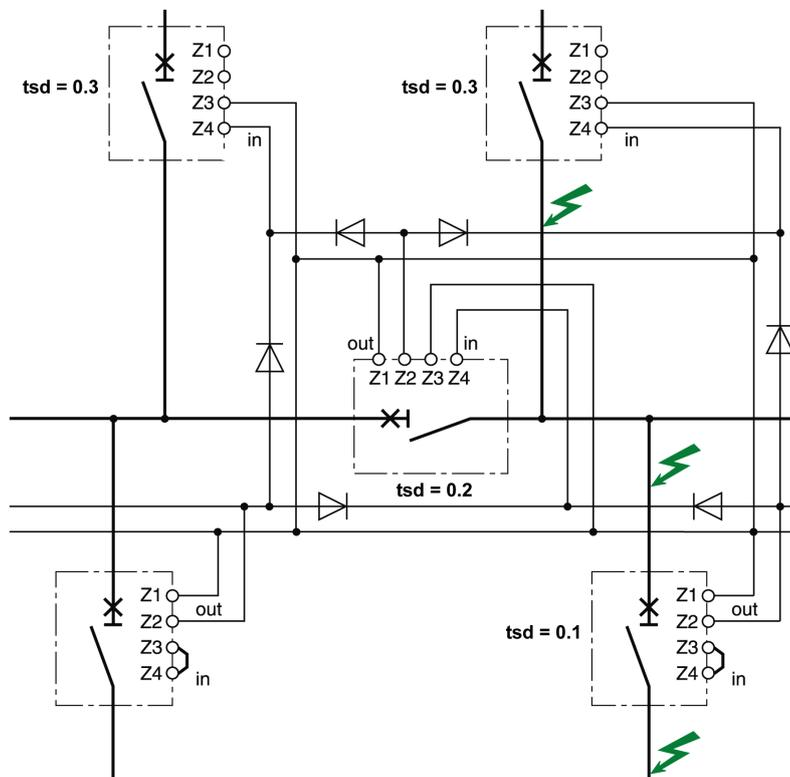
**NOTE:** Management of this configuration does not require any additional relays for ZSI to be controlled for the sources used.
