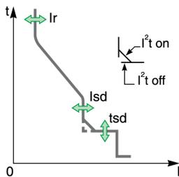
The short-time overcurrent threshold  $I_{sd}$  sets the level of short-circuit current at which the circuit breaker trips when reaching the short-time overcurrent time delay.
