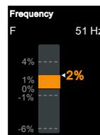
Orange color indicates measurement is out of range: the difference between the measured and expected frequency is between +1% and 4% or between -1% and -6%
