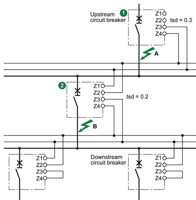
**NOTE:** On circuit breaker 1, the tsd and tg tripping delays must not be set to zero because this would make selectivity impossible.
