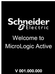
The start-up screen is displayed every time the MicroLogic Active control unit is energized. None of the buttons on the control unit are functional while this screen is displayed. The screen is displayed for the period of the control unit start-up time. At the end of this period, the LSIG home screen or any active pop-up screen is displayed.
