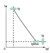
The IDMT ground-fault protection threshold Ig sets the level of ground-fault current at which the circuit breaker detects a ground fault that can lead to a trip, based on a High Voltage Fuse (HVF) tripping curve (I<sup>4</sup>t).
