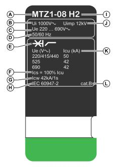
A Circuit breaker size and rated current x 100 A
