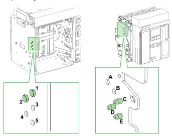
The pin combination selected on the chassis must correspond to the pin combination selected on the circuit breaker (see following table). For example, the combination 12 on the chassis corresponds to the combination CDE on the circuit breaker.
