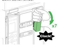
Automatic charge: If the optional MCH gear motor is installed, the spring is automatically charged after closing.
