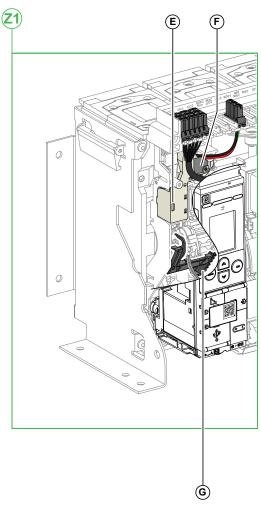
E Standard SDE1 fault-trip indication contact
