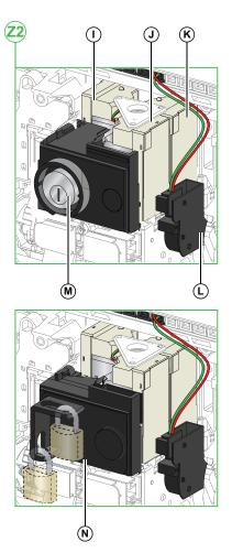
I MN undervoltage release or MX2 opening voltage release
