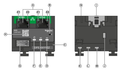
A Two RJ45 Ethernet ports
