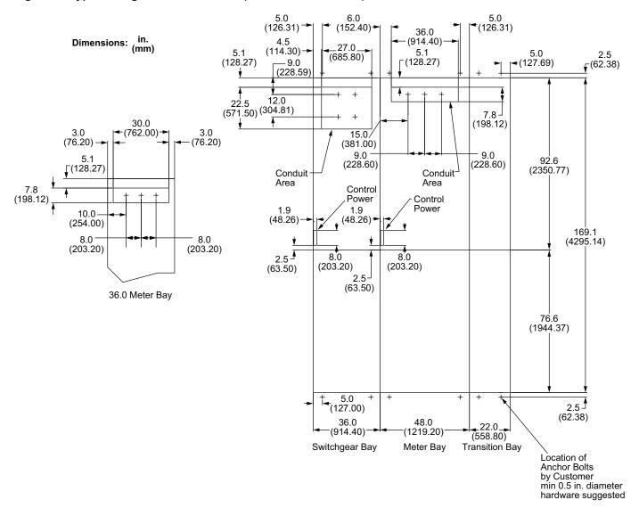
Figure 4 - Typical Common Aisle Floor Plan (Not for Construction)
