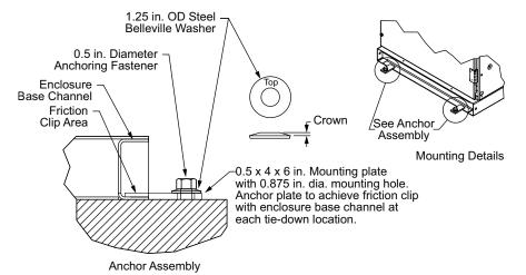
Figure 27 - Non-seismic Switchgear Anchor Assembly
