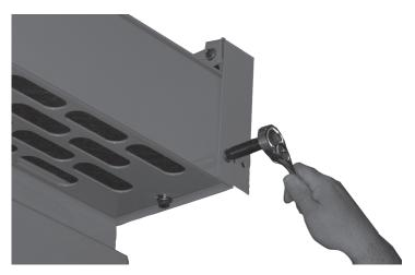
14. Mount the switchgear roof cap to the roof at each end using 1/4 inch threadforming screws, then mount the roof cap to the aisle roof support using two 1/4 inch carriage bolts, seal washers, and locknuts all supplied by Schneider Electric (see Roof Cap Mountings, page 28).
