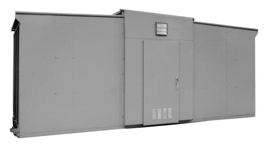
The common aisle switchgear is shipped with the "low side" and the "high side" switchgear sections fully assembled and ready to set on a concrete pad. The aisle is shipped in subassemblies.
