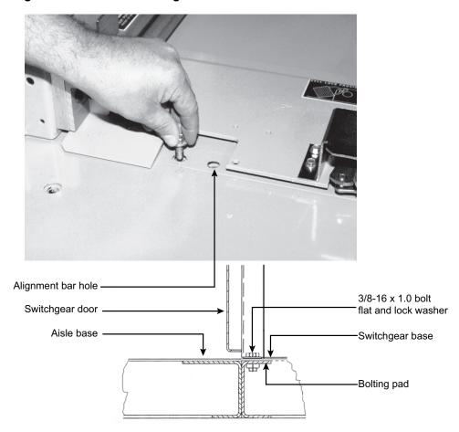
5. After the aisle section is in place and attached to the switchgear section, remove the end shipping braces. Do not remove the braces from in front of the switchgear as it may be necessary to lift the aisle section again if it does not align properly.
