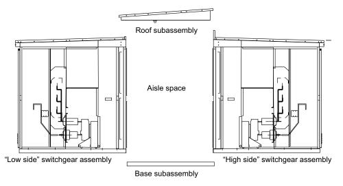
Figure 26 - Common Aisle Configuration
