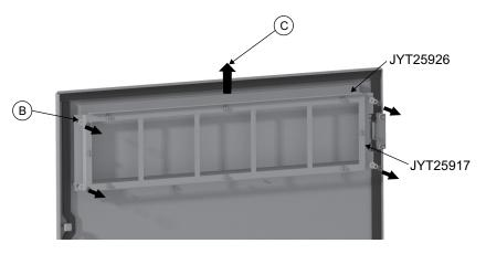
Figure 38 - Replacing the New Filter (Top Louver)
