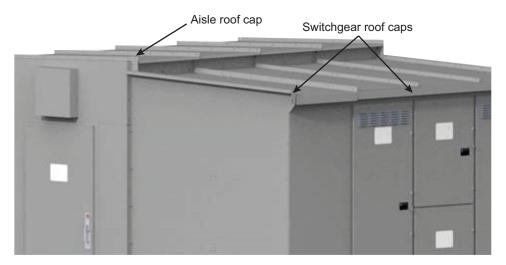
15. Inspect the walk-in switchgear for any openings that may expose the equipment to rain. To do so, enter the walk-in enclosure, close the doors, and look for any light coming through the joints, mainly in the corners (Checking Enclosure for Openings in the Seal, page 28). Make note of them, and seal with caulk. Look mainly for cracks that could be directly exposed to rain.
