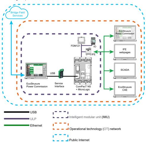
The intelligent modular unit (IMU) represents the MasterPacT NT/NW, ComPacT NS, or PowerPacT P- or R-frame circuit breaker, the MicroLogic trip unit, and the associated ULP modules, communication interface, and IO modules.
