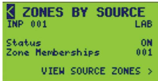
The control source's nametag, status, and zone membership value is displayed on the far right. In the previous screen the control source is a member of one zone. If the control source was not a member of any zones, "000" will appear. See table below for descriptions of the STATUS BY SOURCE screen options.
