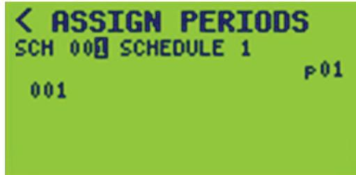
4. Select a period to assign to the schedule by highlighting it and selecting the green (+) button. When a period is assigned to a schedule, its number will be underlined.
