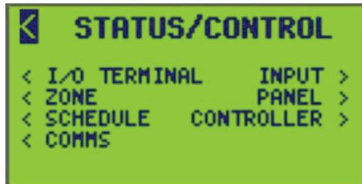
Observable status/control information ranges from the ON/OFF state of sources, number of packet errors regarding protocols used, breakers assigned to panels, timer controls, current analog values from sensors, etc.
