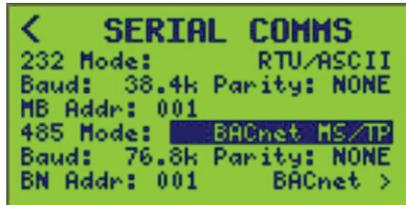
A BACnet access will appear at the bottom of the screen.
