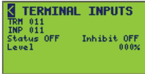
4. If more than one Input Membership, change the input (INP) number to scroll through other inputs that the terminal is assigned to.
