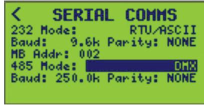
The controller screen will automatically change to show setup fields for the DMX512 mode.
