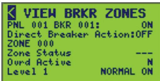
The circuit breaker’s number, panel, actual state, and direct breaker action state with the assigned zone’s status, override state, and priority level are displayed. See Zone Information by Control Source Data, page 86 for descriptions of the control source options.
