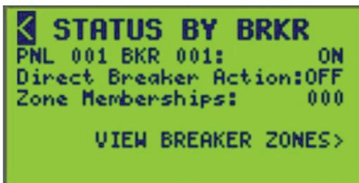
The panel, circuit breaker number, actual circuit breaker state, the direct breaker action, and the number of zones the breaker is a member are displayed. If the circuit breaker was not a member of any zones, then “000” is displayed as shown in the screen above. See table below for descriptions of the STATUS BY SOURCE screen options.
