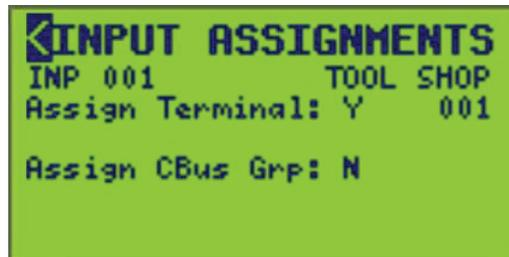
2. Select the input number (INP 001) being assigned to a Terminal, C-Bus Group & Application, or DMX Slot.
