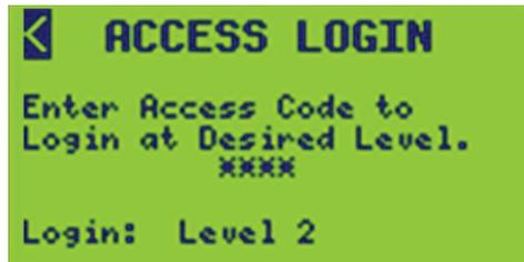
2. Position the cursor over each digit location (\*), using the + or - key to increase or decrease the number to enter the assigned 4-digit access code.
