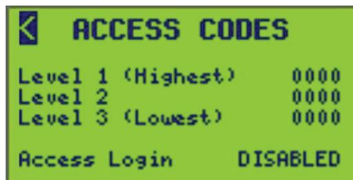
The screen displays the current codes for each of the three levels. The previous screen is the default ACCESS CODES screen.
