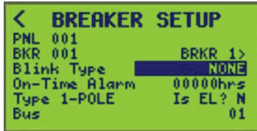
In this screen, the BLINK TYPE for circuit breaker 001 (named BKR 1) on control bus 01 is set to NONE.
