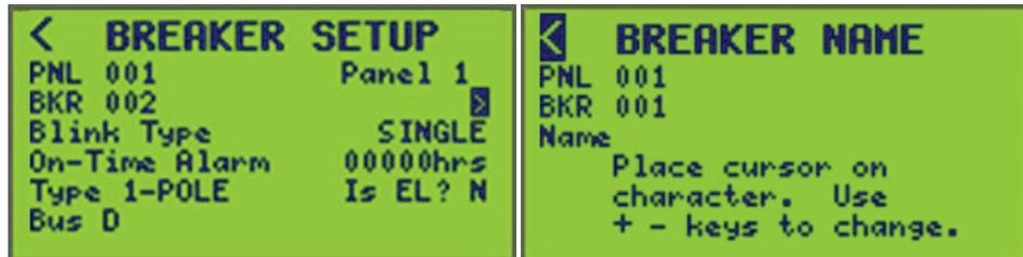
**NOTE:** Verify the desired panel number is selected before assigning or renaming a breaker. Only detected breakers are available when scrolling through breakers (BKR).
