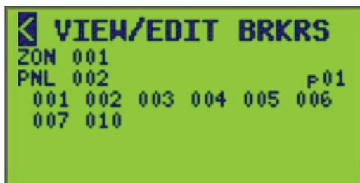
The ZON line displays the selected zone number and nametag from 1–256 (displayed as ZON 001), and the Panel line displays the selected panel number and nametag from 0–7 (displayed as PNL 002). The breakers available on the selected panel are shown below ZON and PNL (maximum 24 breakers per page. See Viewing Circuit Breaker Pages).
