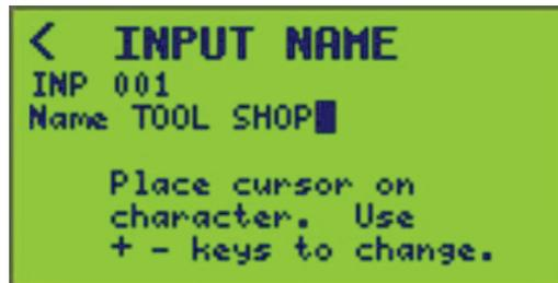
4. To save, press the "<" key and return to the INPUT SETUP screen or change an INP value.
