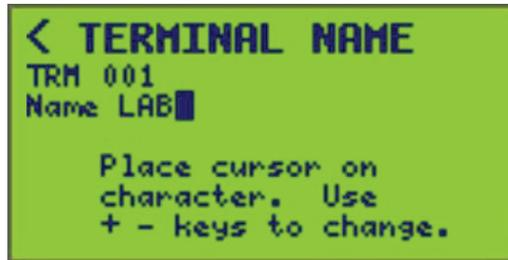
4. To save, exit the TERMINAL NAME screen and return to the TERMINAL SETUP screen or change the TRM number.
