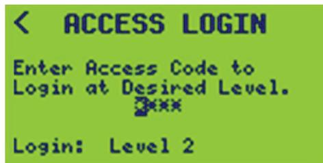
3. Save the code entry by moving the cursor to the exit ACCESS CODES arrow (<) at the top of the screen.
