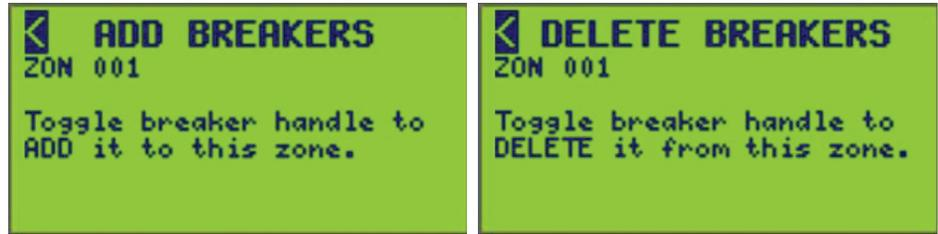
The controller is placed in the LEARN mode upon entering either of these screens. Any circuit breaker that changes state while on the ADD BREAKERS screen or DELETE BREAKERS screen is either ADDED or DELETED from the zone's circuit breaker map.
