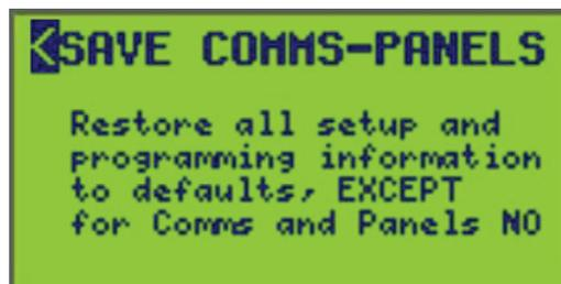
2. Select “YES” to partially restore the controller to factory defaults (excluding the Communications and Panels Configuration).
