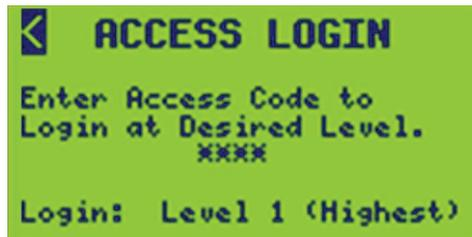
**NOTE:** A five-minute timer restarts every time a key is pressed. When this timer expires, the entered access code is cleared and the user is logged out.
