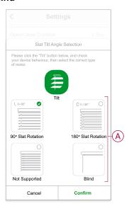
**IMPORTANT:** If the shutter is installed with a non rotating slat or blind, the calibration process is complete, and no further steps to follow.
