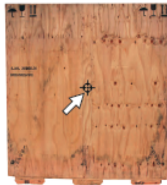
Figure 18 Centre of gravity information on the transport unit (wooden crate for export packaging)
