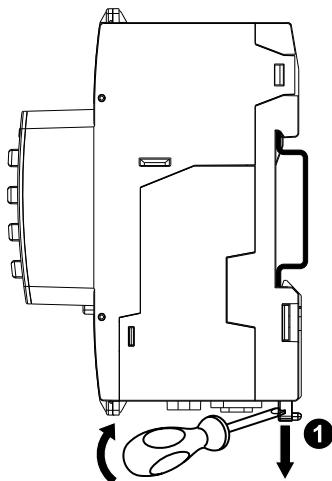
2. Lift the meter out and up to free it from the DIN rail.
