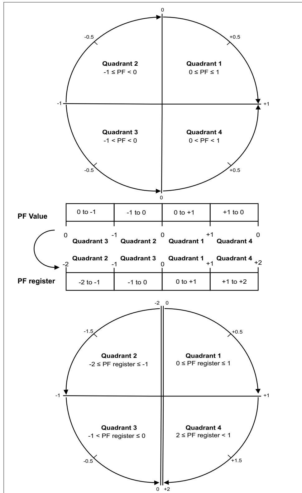
The PF value is calculated from the PF register value using the following formulae:
