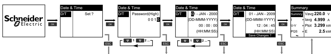
1. Press **OK** when you are prompted to set the date and time when the meter is powered up.
