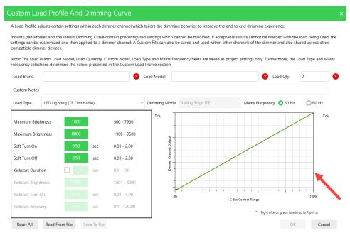
**NOTE:** The Dimming Curve translation is applied after Min/Max scaling, the Min/Max Scaling feature is effectively just limiting the range rather than altering the space of the curve by squashing it over a smaller range.
