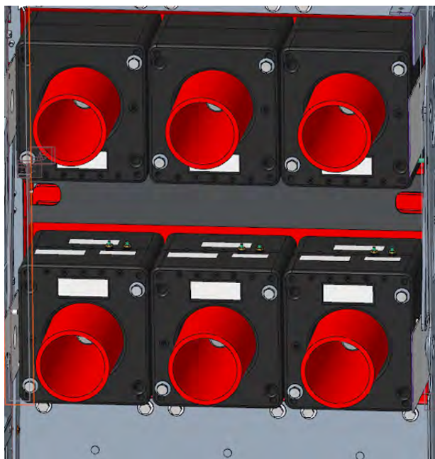
Figure 29 - Current Transformers (2x 348 CTs Per Phase shown)
