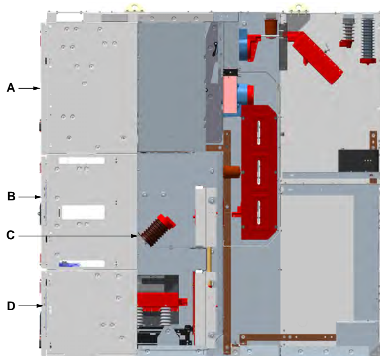
Figure 45 - CPT and LVPT in Position C and D Compartments
